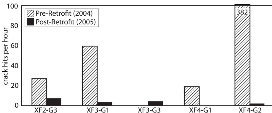
**FIGURE 7.** Crack activity (first hits with amplitude > 55 dB per hour) before and after full retrofit on girder webs G1, G2, G3 and cross frames XF2, XF3, XF4
