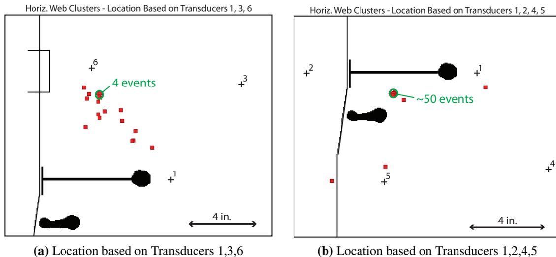
**FIGURE 3.** Alternate cluster analyses on horizontal web. Individual located events are indicated by box icons. Clusters of events are circled.
