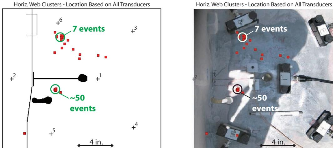
**FIGURE 2.** Clusters of AE events on horizontal web, using location results based on all channels. Individual located events are indicated by box icons. Transducer 2 was used in combined mode; events producing first hits on Transducer 2 were rejected outright, but events producing subsequent hits on Transducer 2 were located. Clusters of events are circled.
