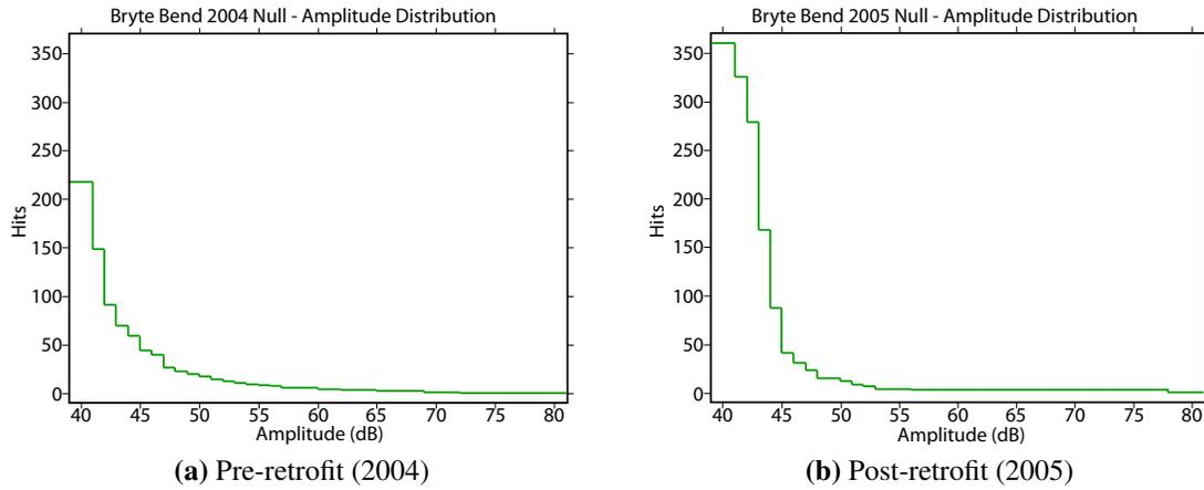
**FIGURE 6.** Amplitude distributions from Bryte Bend pre- and post-retrofit null tests, showing comparable levels of overall AE activity
