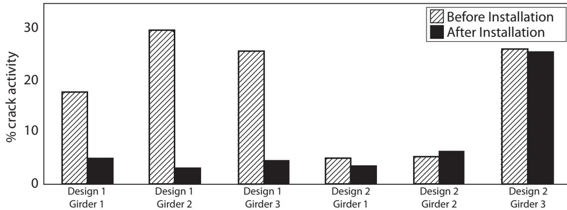
**FIGURE 4.** Crack activity at prototype retrofit sites (modified from Prine and Marron [8])
