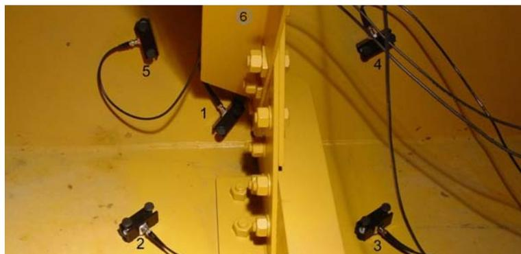
**FIGURE 5.** AE transducer array for first-hit channel analysis of fatigue-prone detail during post-retrofit test
