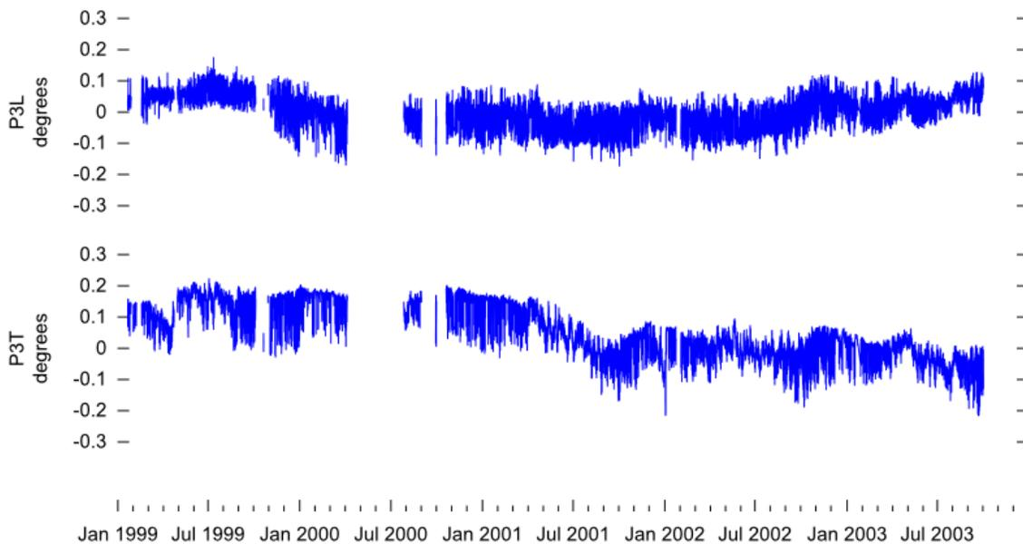
**Figure 4:** Time history of typical longitudinal and transverse response of a pier
