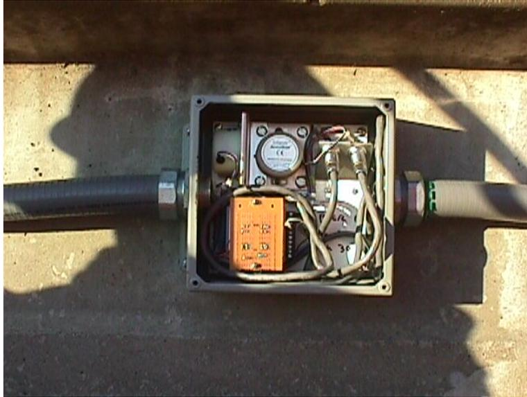
**Figure 2:** Tilt sensor enclosure deployed on bridge. The lid of the enclosure has been removed to show the contents. The orthogonal pair of tilt sensors is visible on the angle bracket in the upper left corner of the box, and the modular electrical connectors are visible at the upper right.
