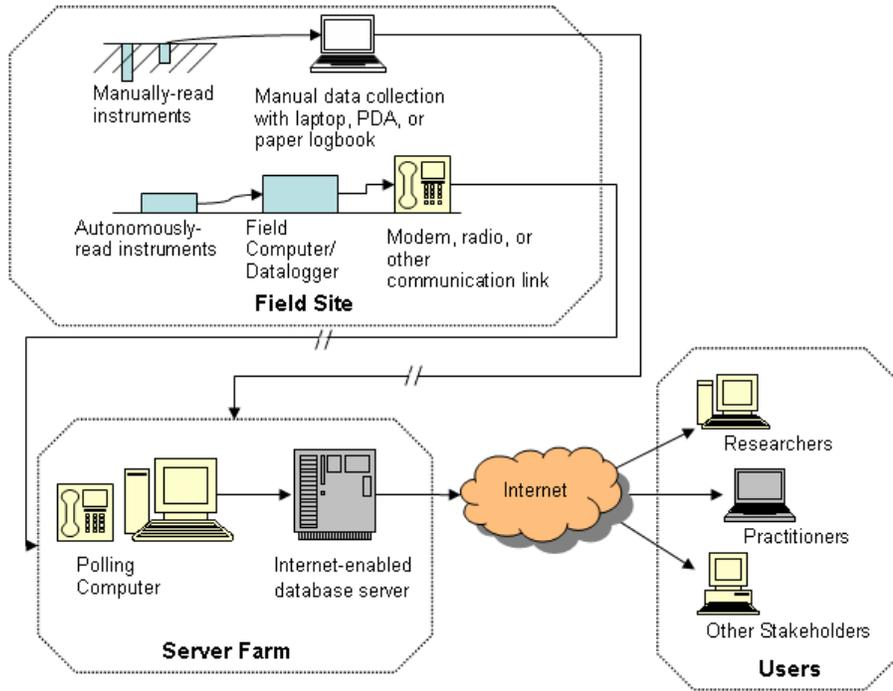
**Figure 3:** Autonomous transmission of data from field to password-protected Web site (after Kosnik <sup>3</sup>)
