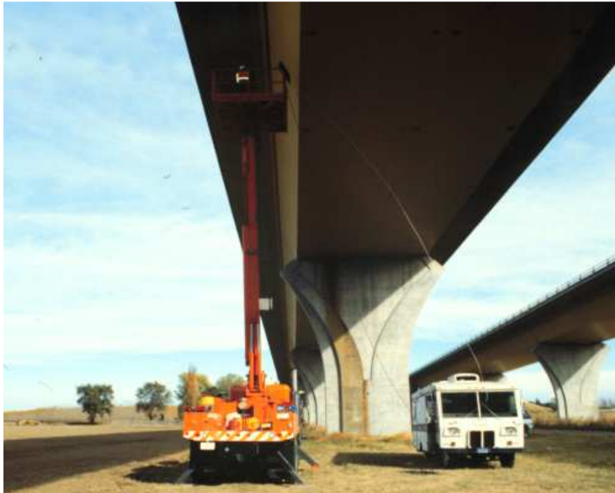
Figure 3. Motor Home Used to House AE Instrumentation.
