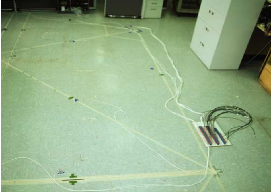
Figure 6. Crossframe Mock Up Used for Wiring Harness Development.
