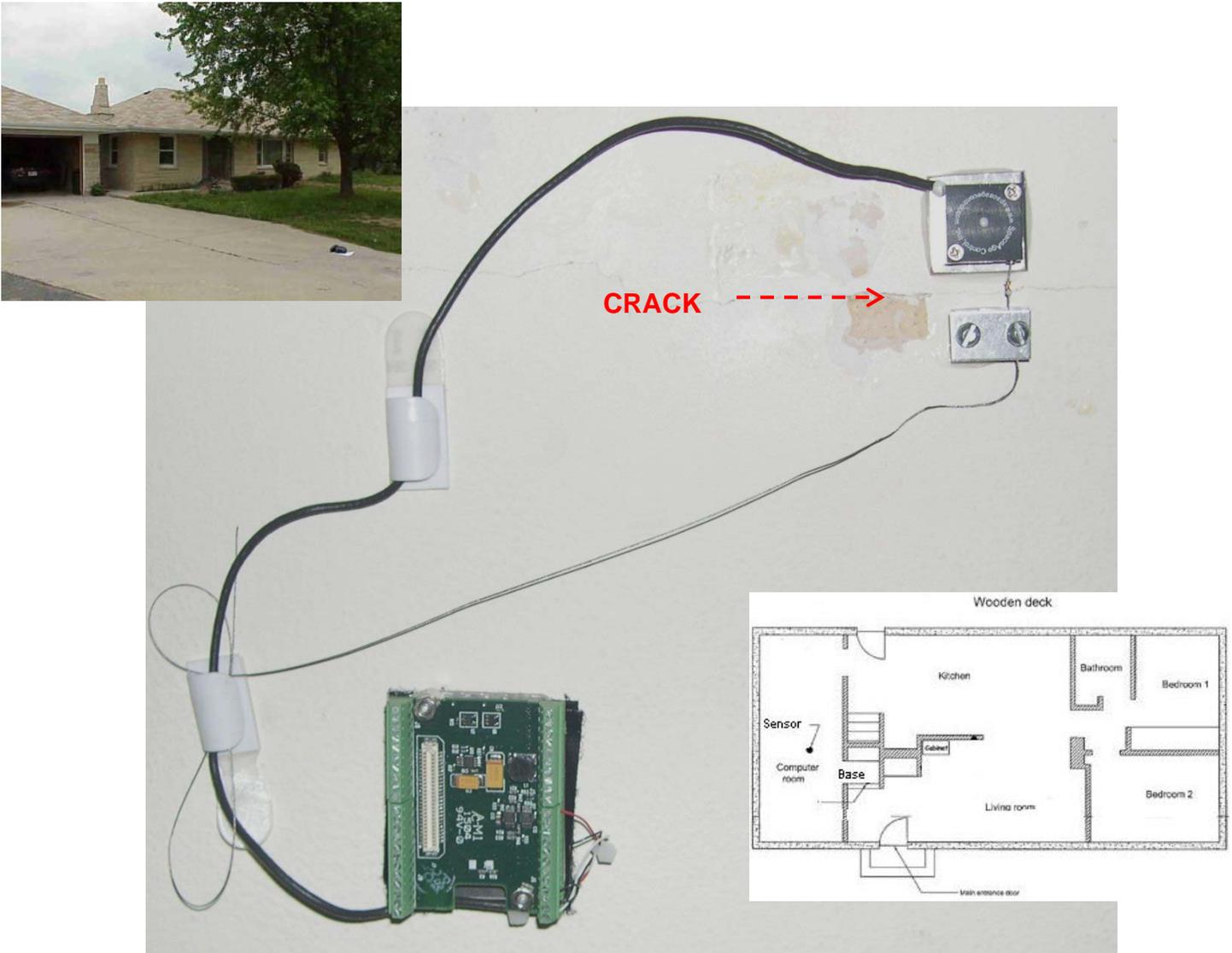
Figure 2: MDA300 and Potentiometer mounted over crack with plan view and picture of house
