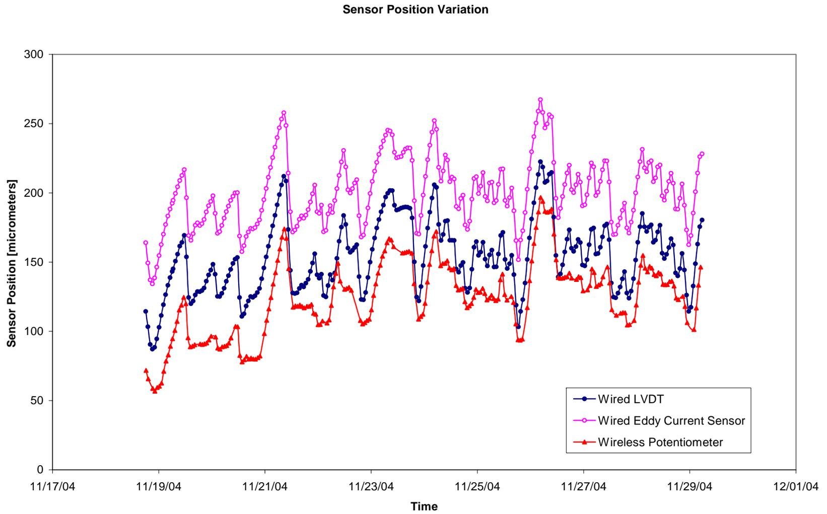
Figure 6: Comparison of Results from wired and wireless data acquisition systems
