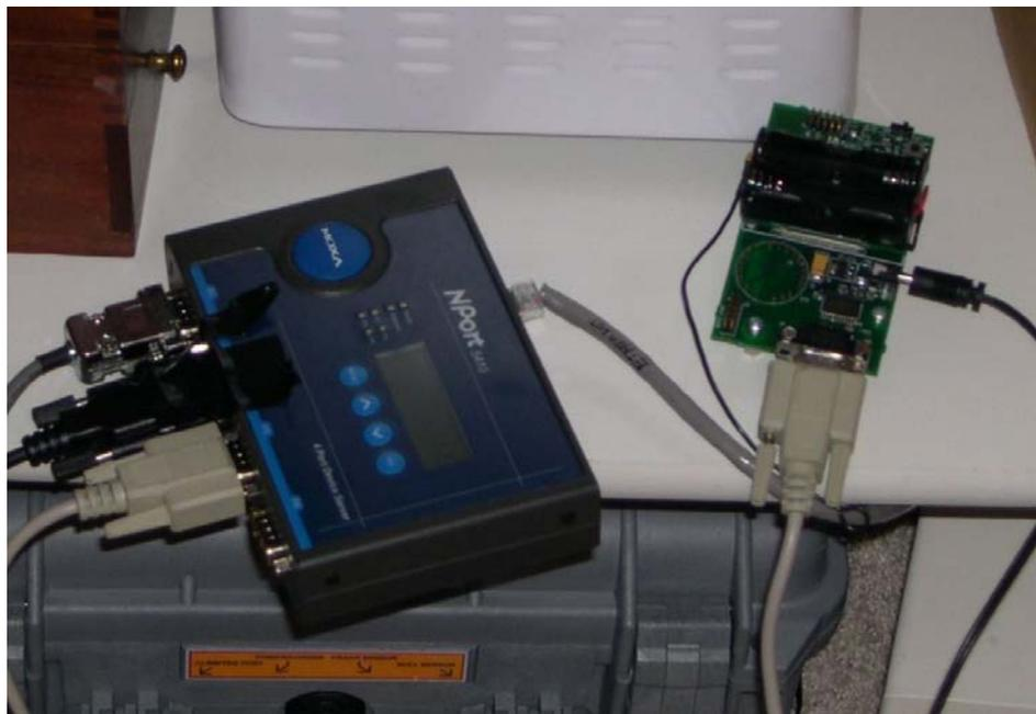
Figure 3: MOXA NPort (left) and MIB510 with mote running TOSBase (right)
