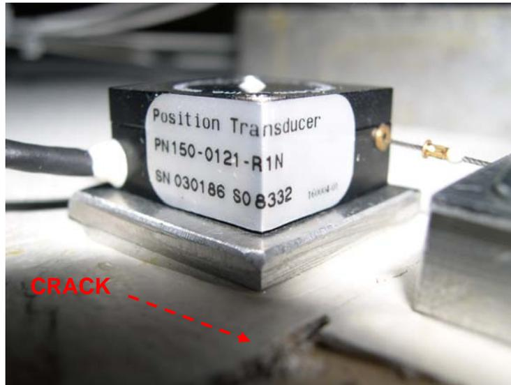
Figure 5: Close-up view of the potentiometer across the crack
