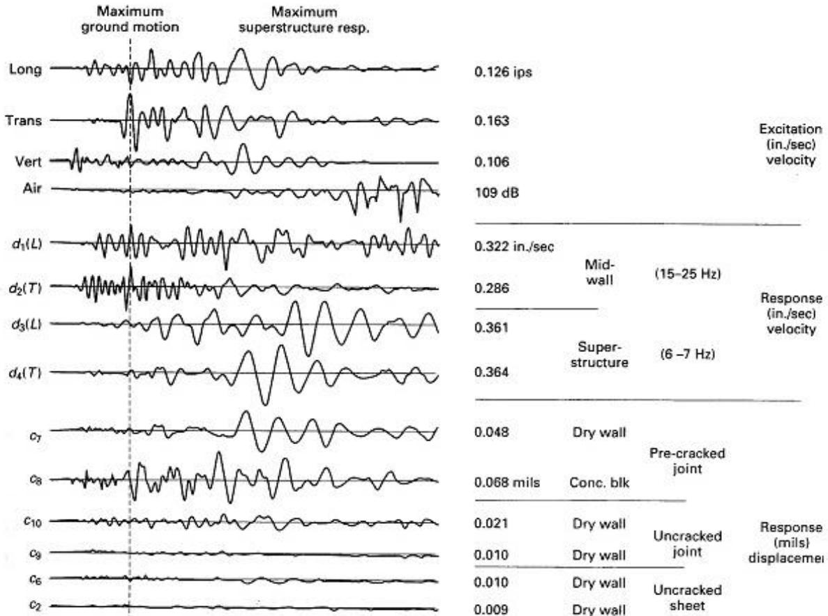
**Figure 7: Response of 14 Transducers to 0.163 ips (4 mm/s) Ground Motion That Shows Wall Response to the Early Arriving High Frequency Motions and The Later Arriving Low Frequency Waves.**
