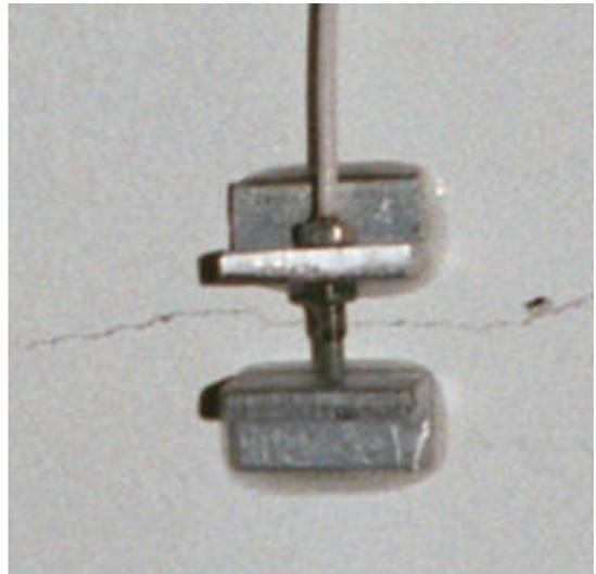
**Figure 2: (Left) Eddy Current Sensor Across Hairline Crack in Dry Wall Joint at Door Corner. This Device Can Measure both long-term and Vibratory Changes in the Crack Width. (Right) Enlargement of a Second Generator Sensor Target Spanning Cracking in Dry Wall Ceiling Joint.**
