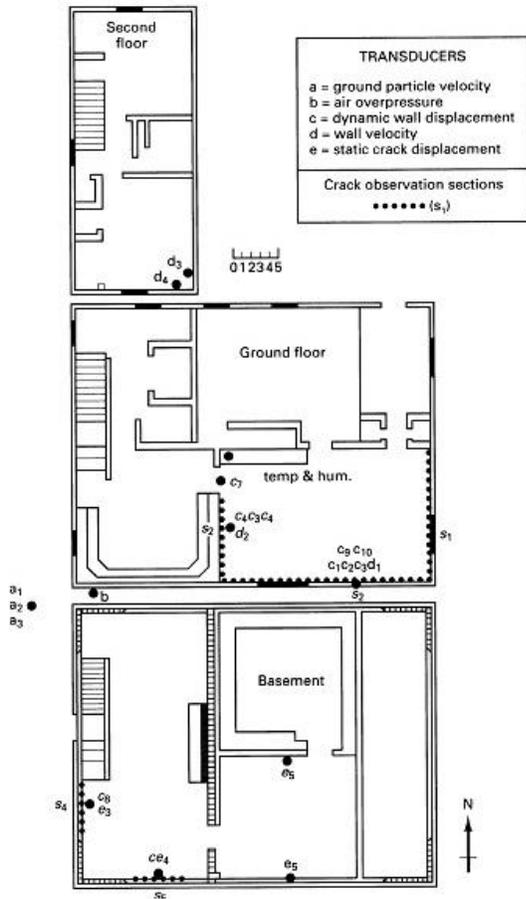
**Figure 5: Plan View of House Showing Transducer Locations.**
