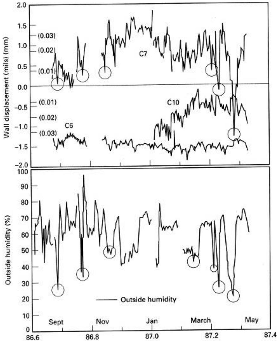
**Figure 8: Eight Month History of Displacement and Crack Displacement Showing Greatest Change in Crack Width to Correlate with the most Intense and Longest Drop in Humidity in April.**
