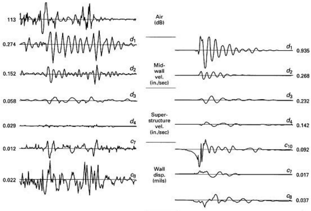
**Figure 6: Comparing Velocity and Crack Displacement Response to Thunder and Door Slamming.**
