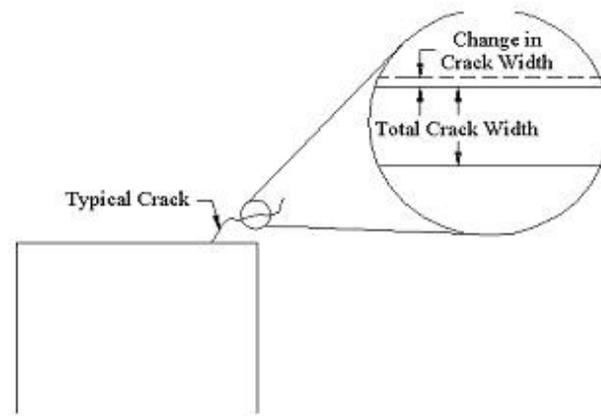
**Figure 3 Micro-Inch Crack Width Change Measured by Eddy Current Sensors.**
