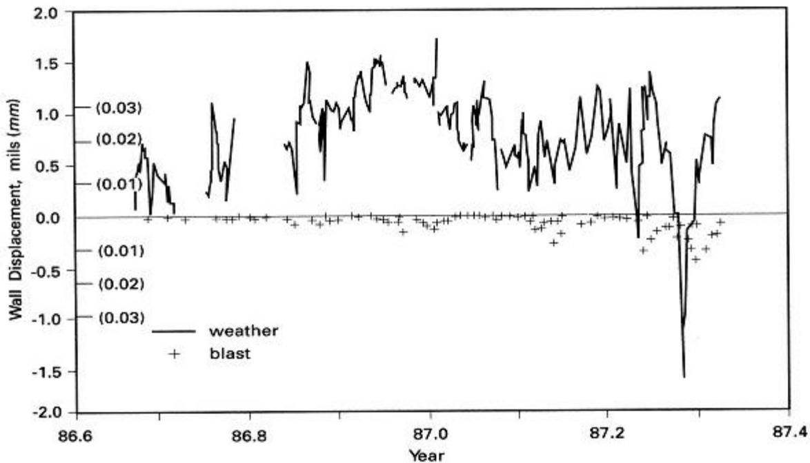
**Figure 9: Comparison of Long-Term and vibration Induced Crack Displacement Showing that the Largest Ground Motion ("+" at arrow) of 0.75 ips (19 mm/s) Produced a Crack Displacement Less Than That of the Passage of a Typical Weekly Weather Front.**
