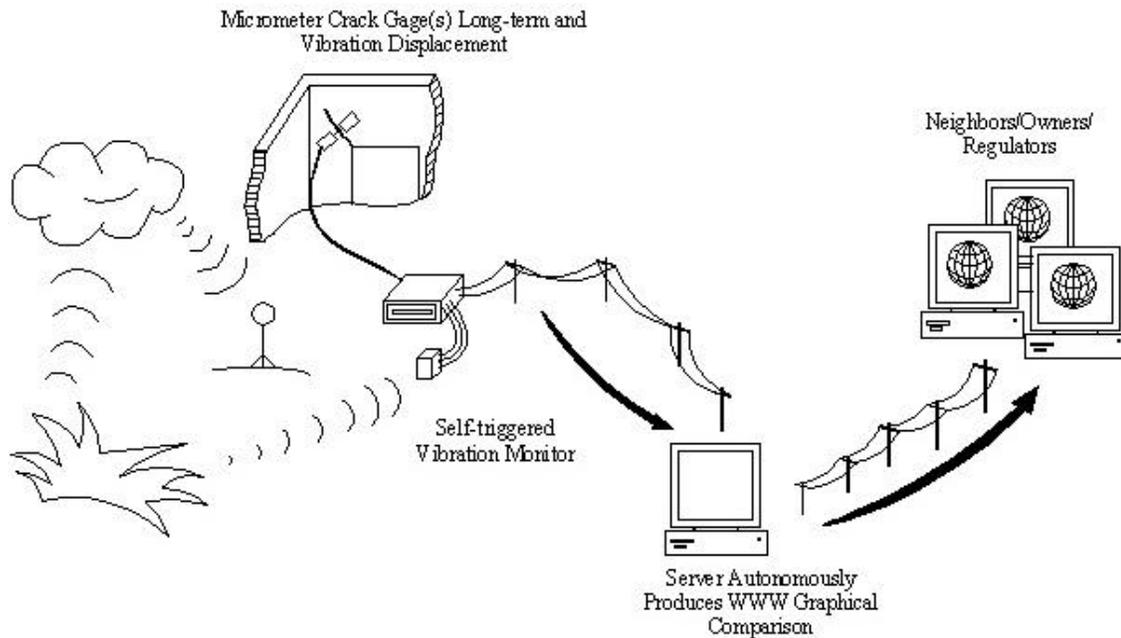
**Figure 10: Autonomous Crack Measurement System Automatically produces graphical comparisons of vibration and environmentally-induced crack displacement, which are accessible to interested parties via the Internet.**
