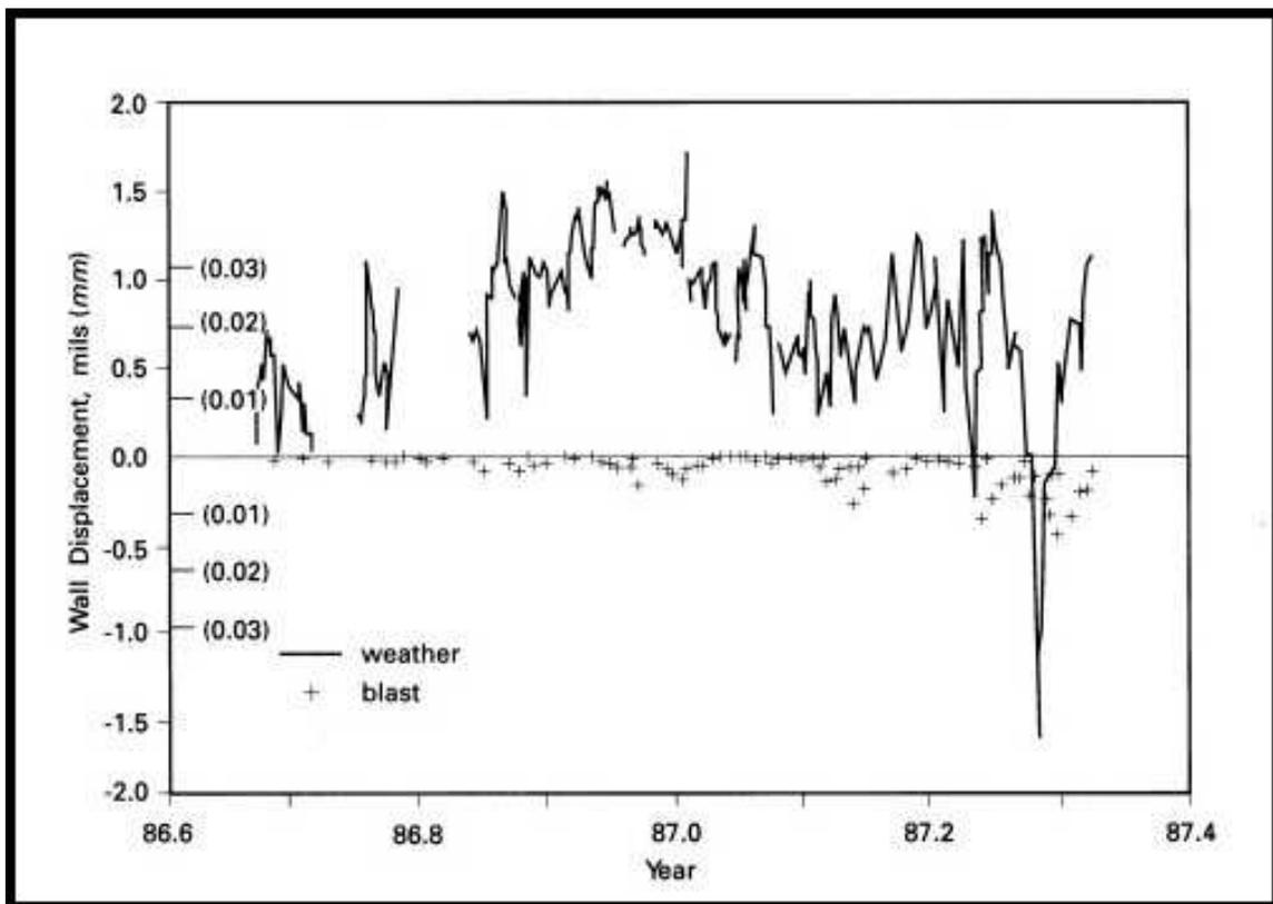
**Figure 4 - Comparison of long-term (silent) weather induced crack response to that from blasting.**
