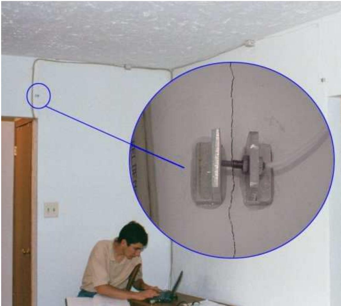
**Figure 1 - Typical instrumented room with detail of crack and sensor**
