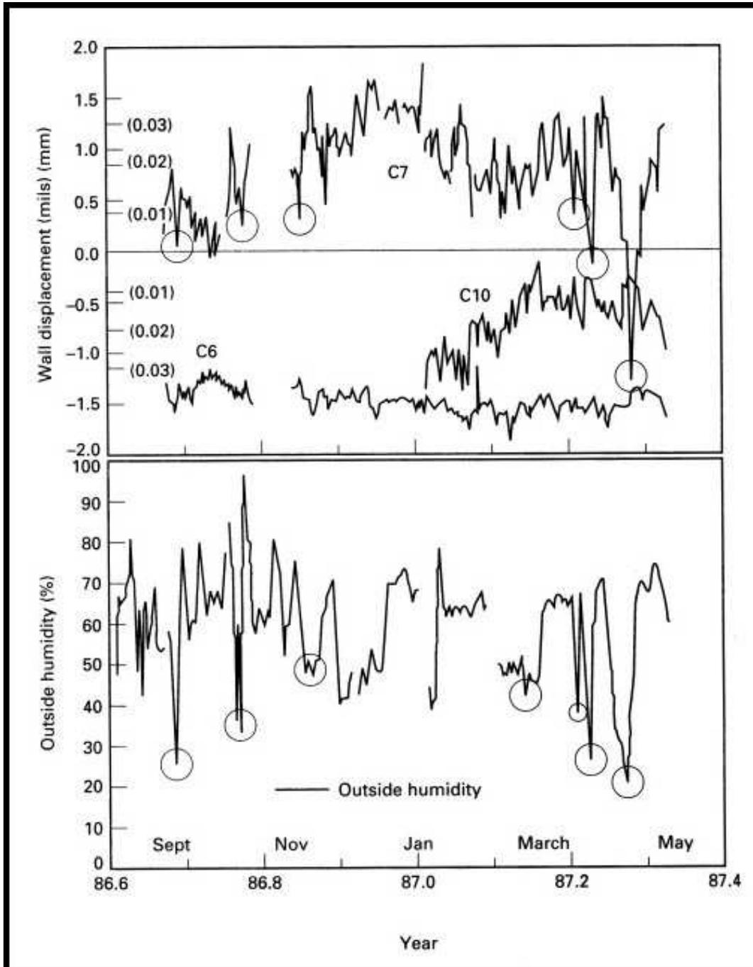
Figure 3 - Comparison of displacement response of cracked tape joint (c7), un-cracked dry wall (c6) and un-cracked tape joint (c10) with changes in outside humidity.
