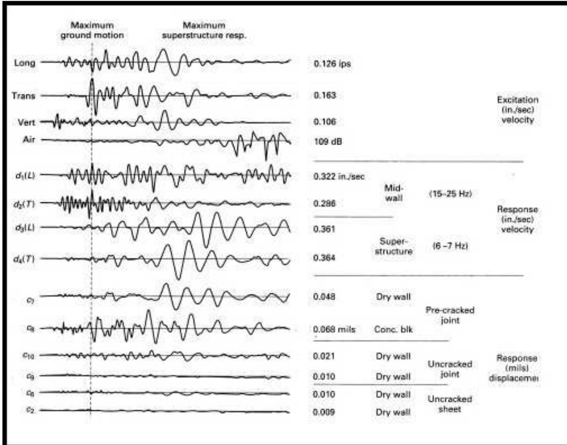
**Figure 2 - Time histories of ground motions, as well as house and crack response from a typical blast.**
