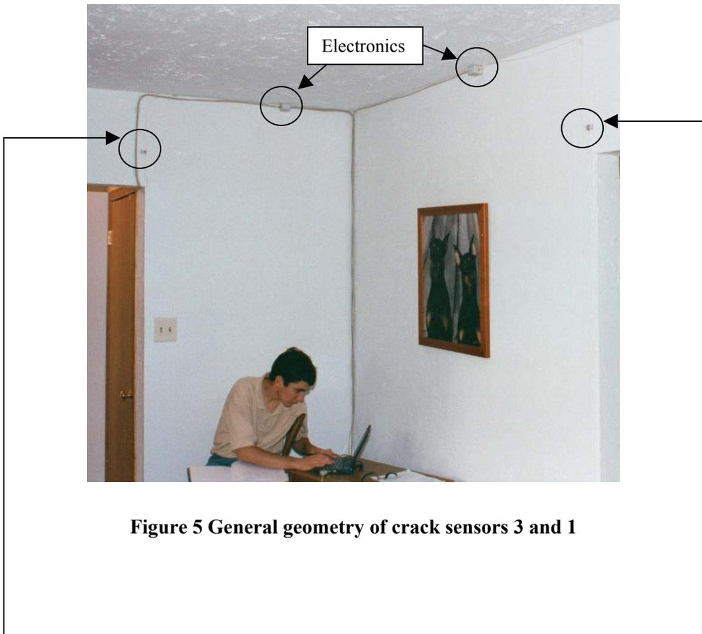
**Figure 5 General geometry of crack sensors 3 and 1**
