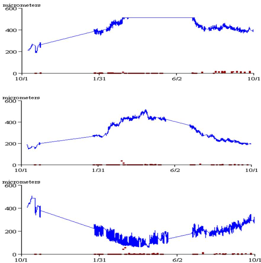
**Figure 11: Year-Long and Vibratory Crack Response Comparisons Shows that Long-Term Effects Are an Order of Magnitude Greater than the Maximum Vibratory Effects. Top: Crack 3. Bottom: Crack 2.**
