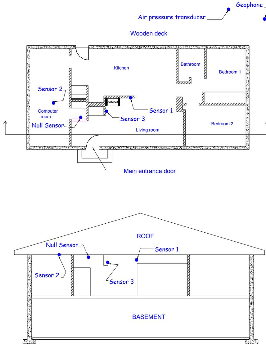
**Figure 4 Plan and Elevation views of the test house**
