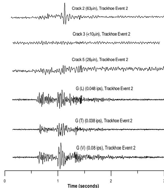
particle velocities (PPV) between 0.03 and 0.456 inches per second and maximum crack response up to 450 micro-inches ( 11 micro meters). Chain trenching produced the least vibration at the test house and will not be discussed in this article.
