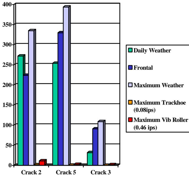
**Figure 5 Comparison of Crack Displacements from Maximum Weather (Tall Bars) and Construction Vibration Effects (Short Bars) for Cracks 2, 3 & 5**
