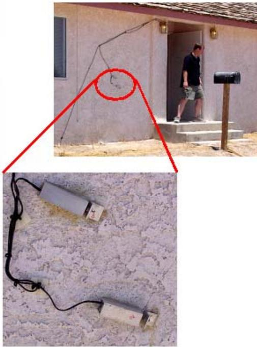
**Figure 1 Test House Showing Closeness of Construction and Sensor Across Crack 2**
