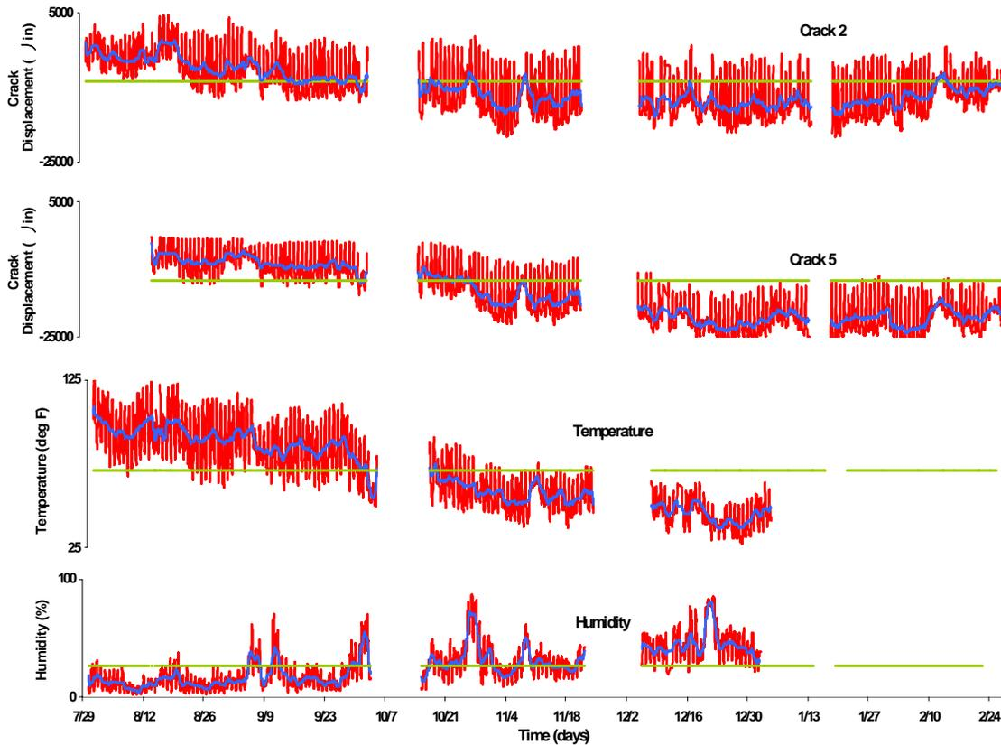
the cracks. The interior of the house is air-conditioned, which controls temperature and humidity, which thus reduces weather fluctuations and crack displacements relative to those outside.
