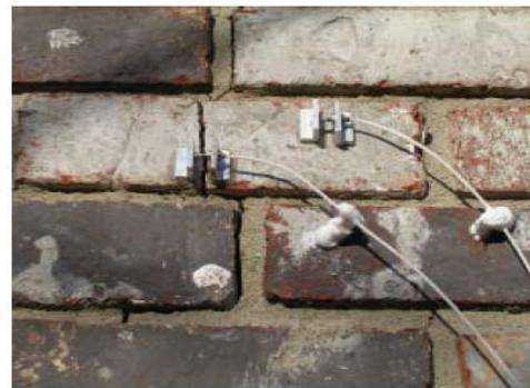
**Figure 2: Orientation and detailed photographs of cracks and sensors for cracks in interior bedroom drywall, basement CMU mortar and exterior brickwork**
