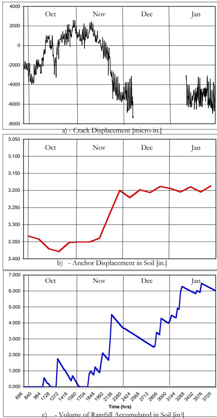
Figure 5: Comparison of crack response (top) with distance between bolts, which indicates swelling when the distance declines (middle) and a crude estimate of the volume of retained water in the shallow soils (bottom). Retained water is the sum of wetting by measured rainfall and drying by estimated evaporation and downward percolation. See Appendix for details.
