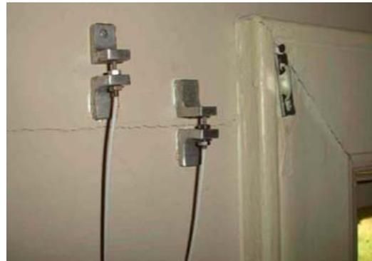
Figure 2: Crack in the interior gypsum drywall showing crack sensor and null sensor.
