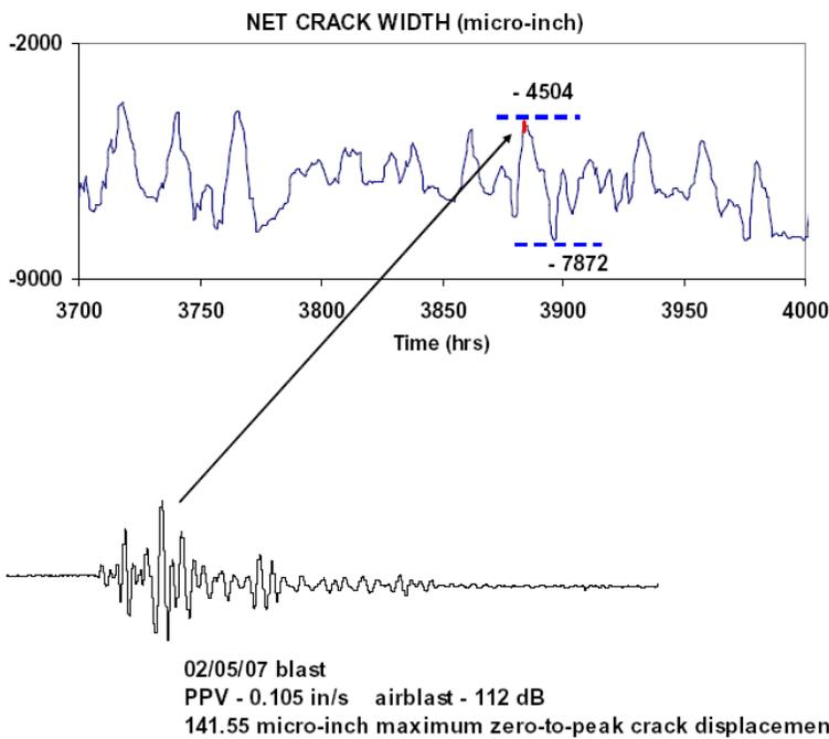
Figure 7 Compares the daily diurnal changes in crack response before and after the 02/05 blast that produced the 2.7 mm/s (0.105 ips) PPV motion showing how large is just the daily crack responses compared to the vibratory responses.
