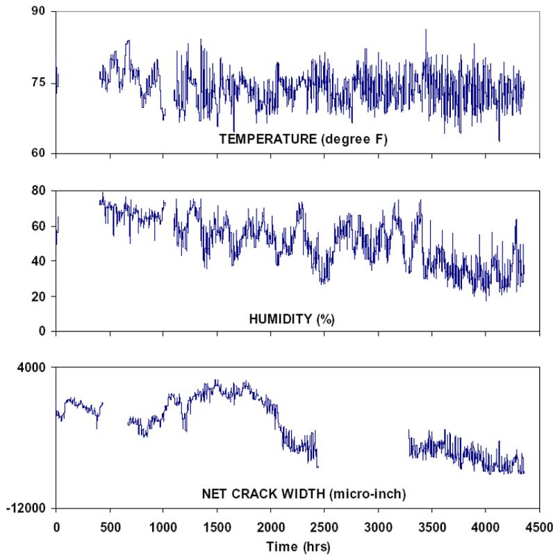
Figure 3 - left: Response of the crack in Figure 2 (bottom) compared to the variations in outside temperature (top) and outside humidity showing large change at 2000-2500 hours (80-100days)
