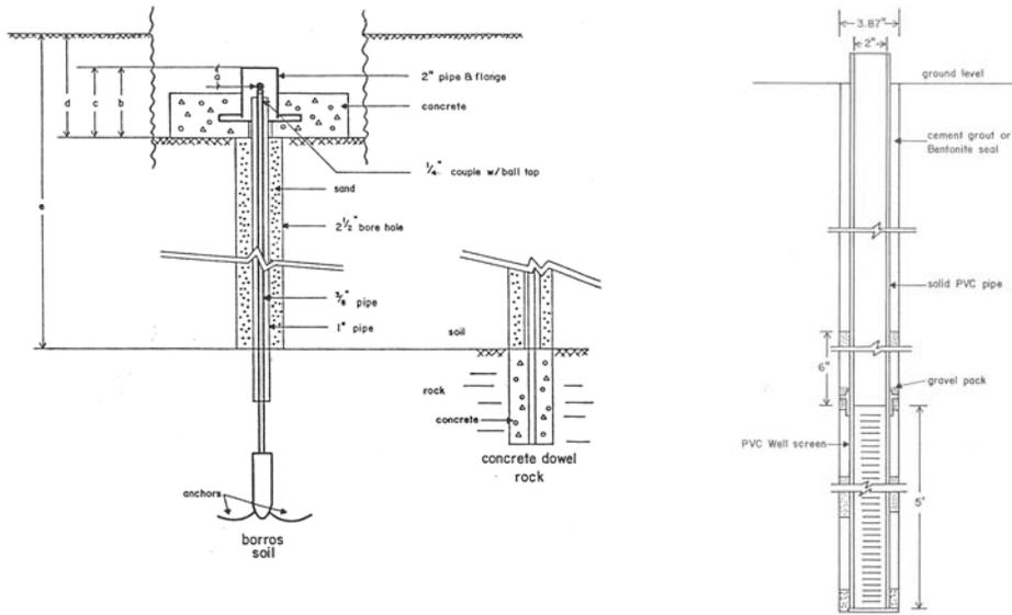
Figure 10: Other versions of inexpensive anchor systems and well for observing changes in the water table. Borros point (left) and rock dowel (center) and PVC well (right).
