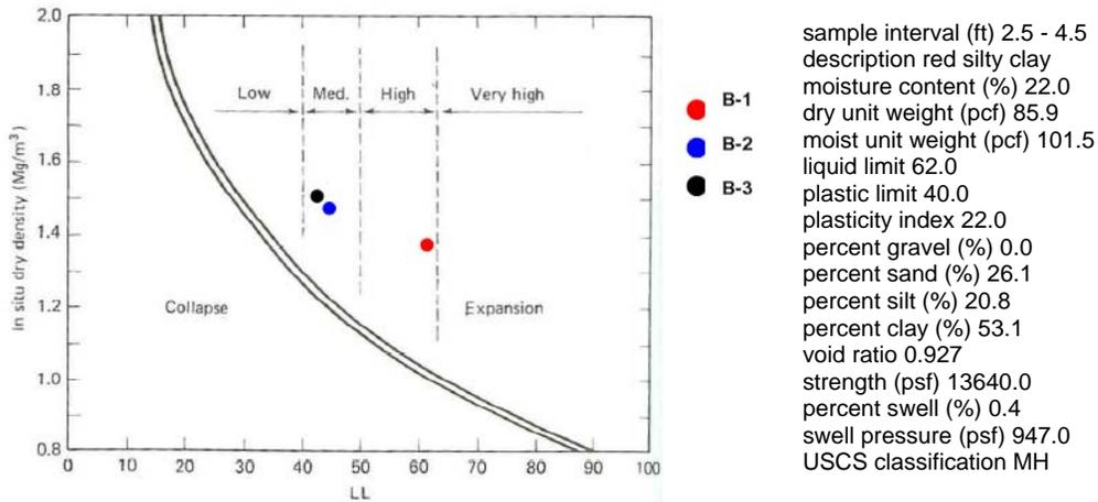
Figure 6: Comparison of soil properties at B-1 the test site with other nearby soils shows those at B-1 to indicative of a soil with a high swell potential(after Holtz and Kovacks, 1981) . A complete soil analysis accompanies the figure on the right.
