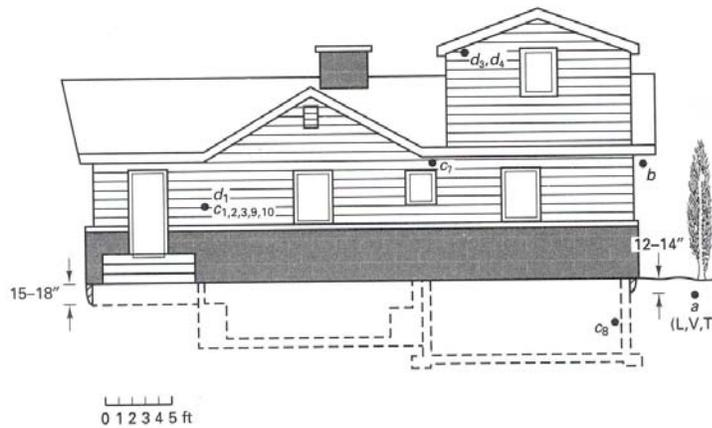
Figure 9: House associated with garage showing the variable foundation depths. The shallowest founded portion (left) displayed the most response to moisture induced volume changes in the soil.
