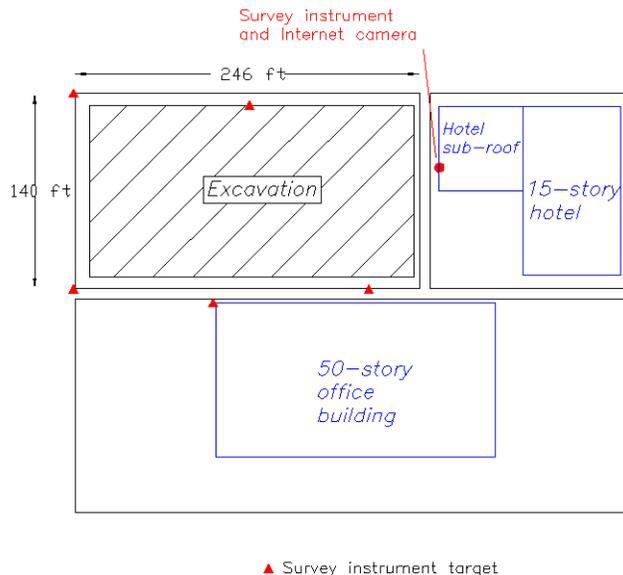
**FIG. 3. Plan view of excavation monitored by automated survey station**
