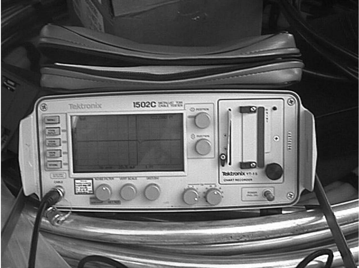
*Figure 1. TDR cable tester; shown with X-Y recorder that can be interchanged with a serial communications port for acquisition of digital TDR traces. The negative spike TDR reflection in the middle of the screen is created by a crimp in the cable being interrogated.*
