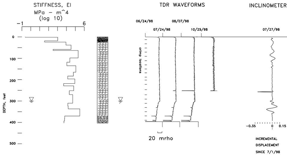
**Figure 3-TDR waveforms and inclinometer profile indicating rock deformation beneath road adjacent to quarry.**
