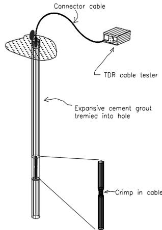
**Figure 1-Schematic of cable installation and monitoring.**
