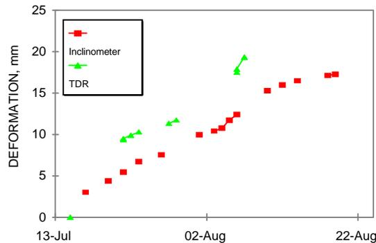
**Figure 4-Comparison of TDR and inclinometer deformation time histories.**
