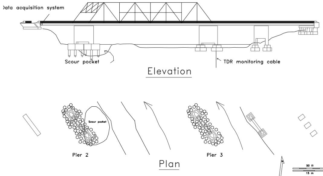
**Figure 2-Overall view of bridge; TDR monitoring cable was installed in Pier 3.**
