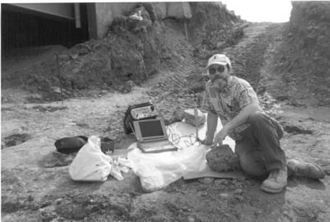
*Figure 2. Interrogating cable with cable tester. Cable was installed to monitor abutment slope movement.*
