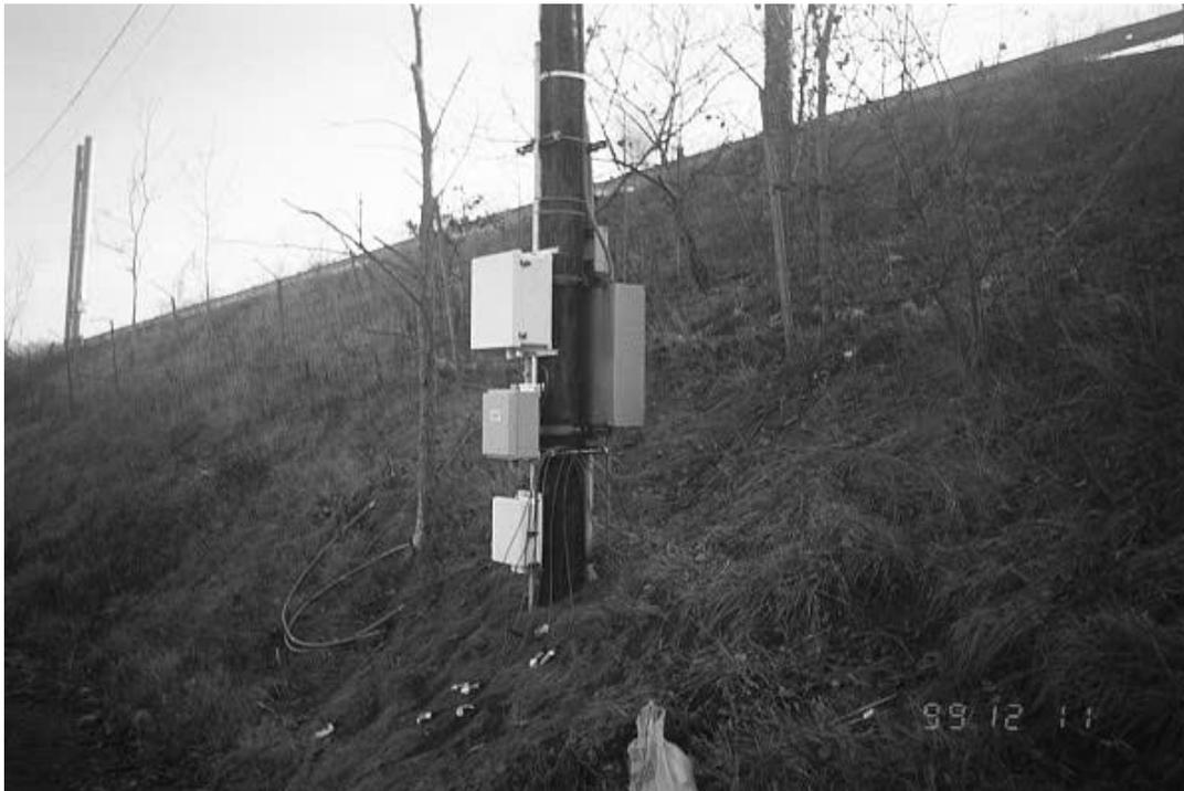
*Figure 4. Remote system installed to monitor subsidence along a highway over an active coal mine.*
