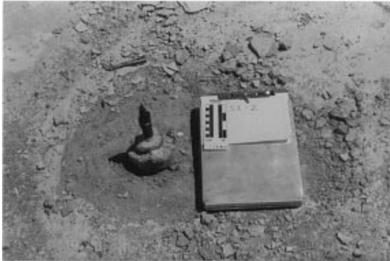
Figure 13. Inclinometer casing retrofitted with grouted coaxial cable.
