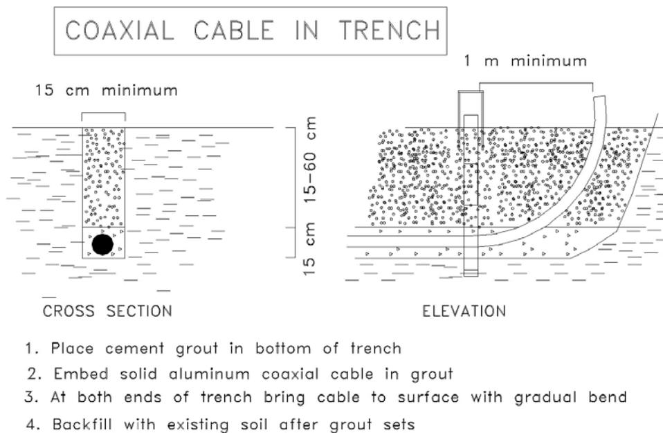
Figure 3. Installation details for horizontal TDR-5 cable, SR 66, Highlands County.
