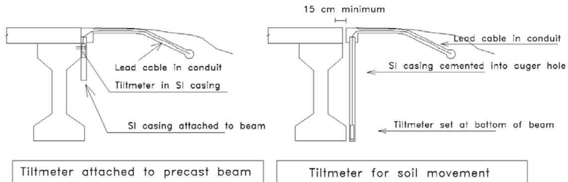
Figure 4. Cross section of the precast concrete beams and installation details for tiltmeters, SR 66, Highlands County, Florida.
