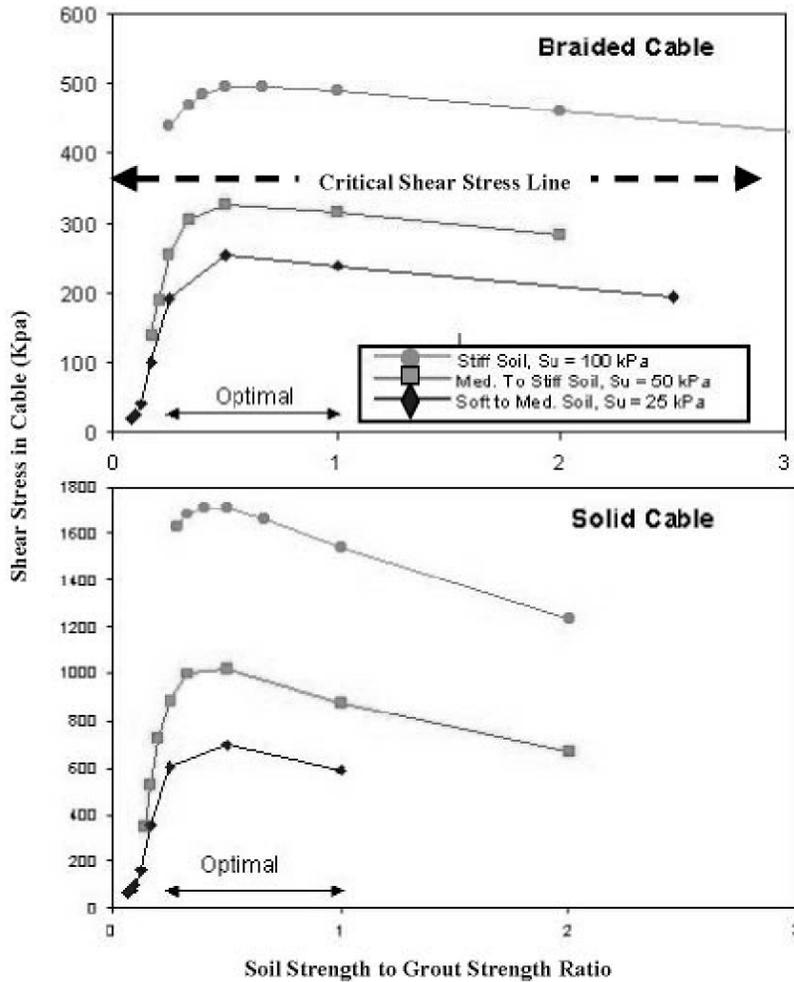
Figure 10. Cable shear stress vs. soil strength to grout strength for solid & braided outer conductor cables (Blackburn, 2002).
