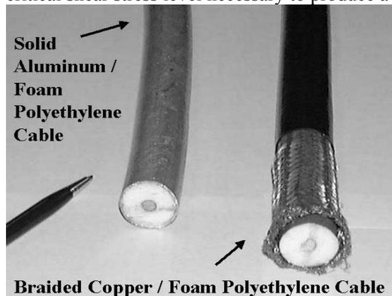
Figure 9. Two most common types of coaxial TDR sensor cables.
