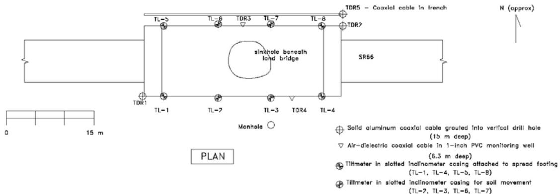
Figure 2. Plan view of the installed instruments (TDR & Tiltmeters), SR 66, Highlands County, Florida
