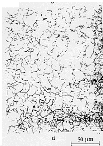
Figure 4. Microstructure of NUCu-Oregon Steel. a - plate A2 as-recieved; b - plate A2 heated at 1250°C for 30 min.; c - plate C1 as-recieved; d - plate C1 heated at 950°C for 30 min.
