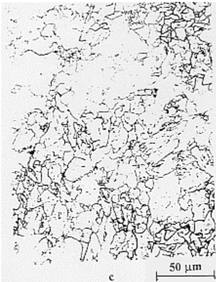
Figure 4. Microstructure of NUCu-Oregon Steel. a - plate A2 as-recieved; b - plate A2 heated at 1250°C for 30 min.; c - plate C1 as-recieved; d - plate C1 heated at 950°C for 30 min.
