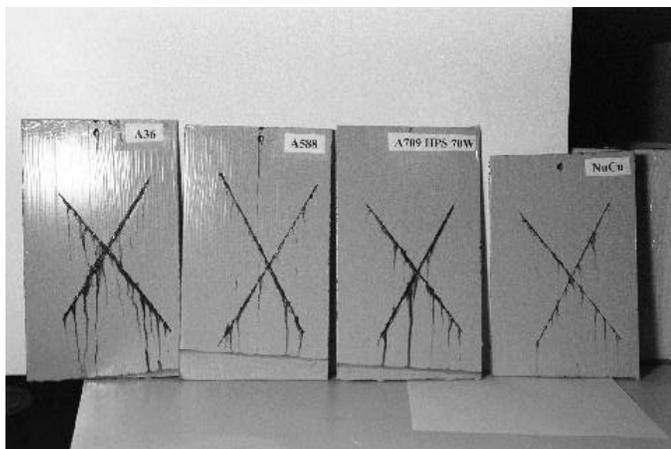
Figure 3. Painted steel panels after 3 weeks, 35°C exposure in salt-fog chamber (A36; A588; ASTM HPS70W; NUCu (ASTM A710 Grade B) steels)
