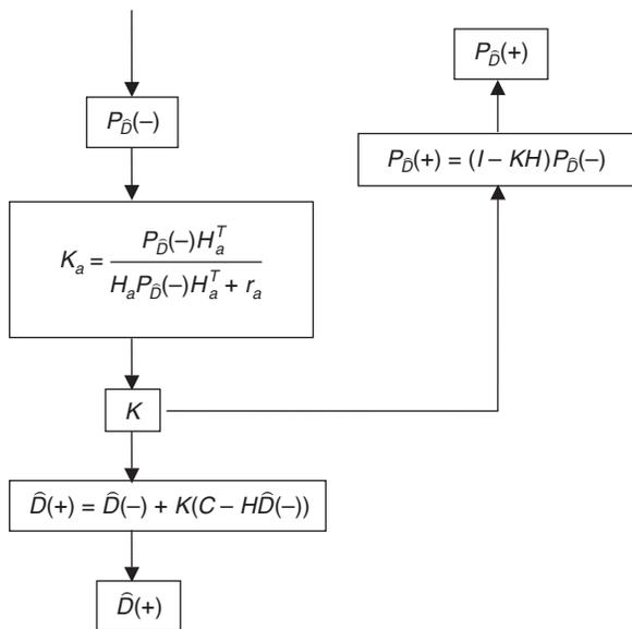
FIGURE 6 Sensor location problem sequential algorithm flowchart.
