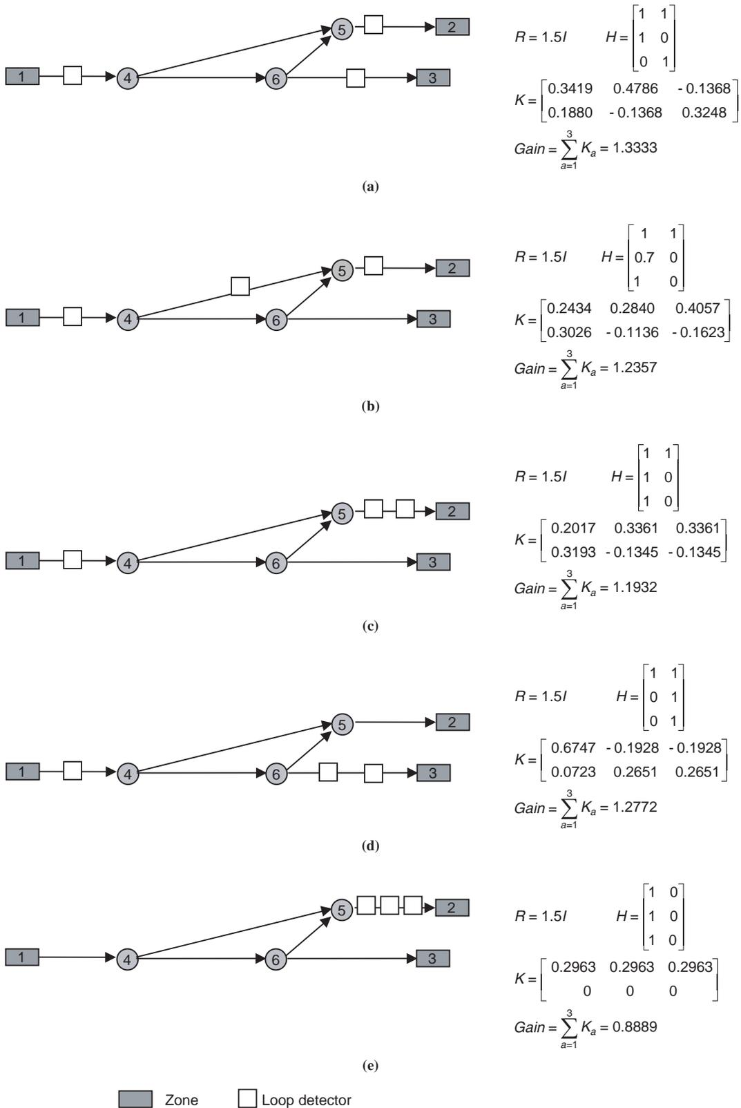
FIGURE 10 Three-point sensor locations: (a) three uncorrelated sensors for both O-D pairs, (b) three uncorrelated sensors for both O-D pairs, (c) three uncorrelated sensors for both O-D pairs, (d) three uncorrelated sensors for both O-D pairs, and (e) three uncorrelated sensors for O-D pair (1-2).
