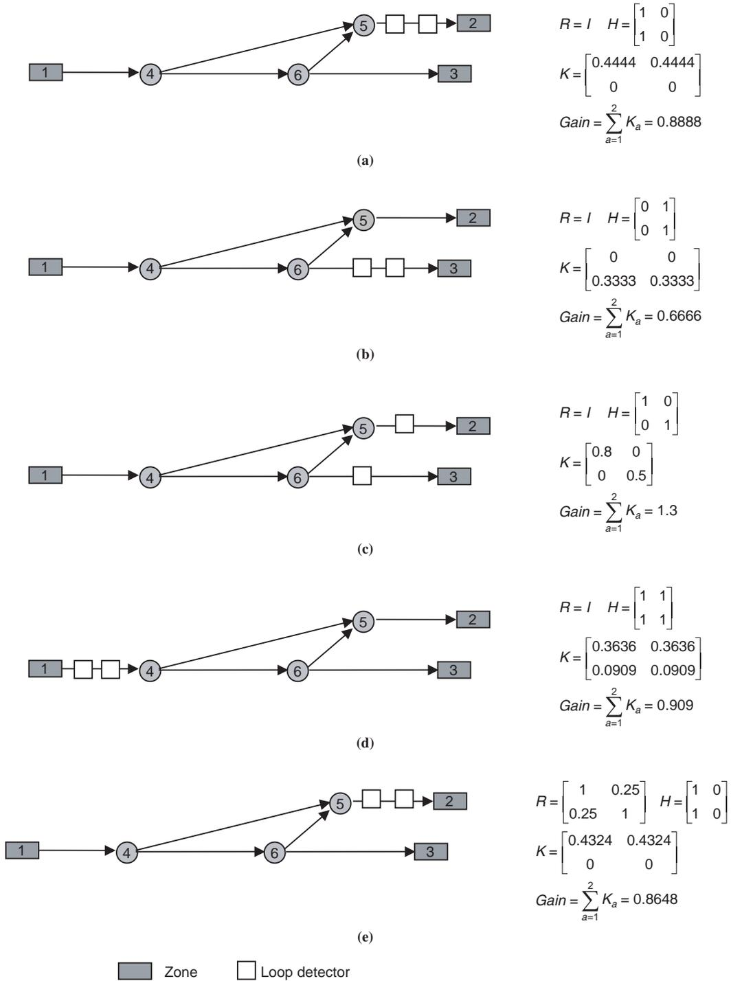
FIGURE 9 Two-point sensor locations: (a) two uncorrelated sensors for O-D pair (1-2), (b) two uncorrelated sensors for O-D pair (1-3), (c) two uncorrelated sensors for both O-D pairs, (d) two uncorrelated sensors for both O-D pairs, and (e) two partially correlated sensors for O-D pair (1-2).
