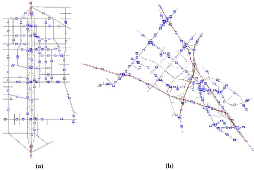
FIGURE 1 Sensor locations by DTA in (a) Fort Worth network and (b) Irvine network.
