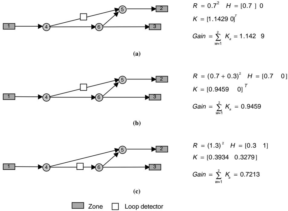
FIGURE 8 Single-point sensor locations with route choice: (a) assignment error-free with link proportion 0.7, (b) standard of link proportion estimation errors (from traffic assignment) = 0.3, and (c) assignment error-free with link proportion of 0.3.
