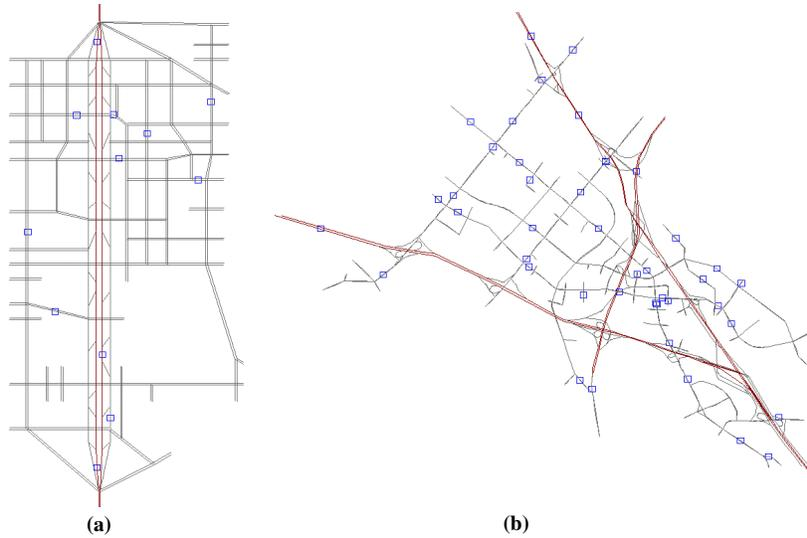
FIGURE 2 Sensor locations by static model in (a) Fort Worth network and (b) Irvine network.
