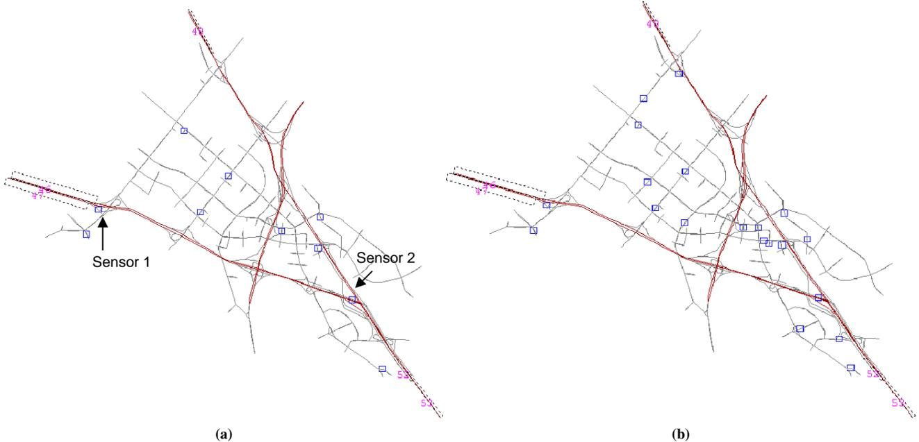
FIGURE 11 Sensor locations by link gain selection in Irvine network: (a) 10 sensors and (b) 20 sensors.
