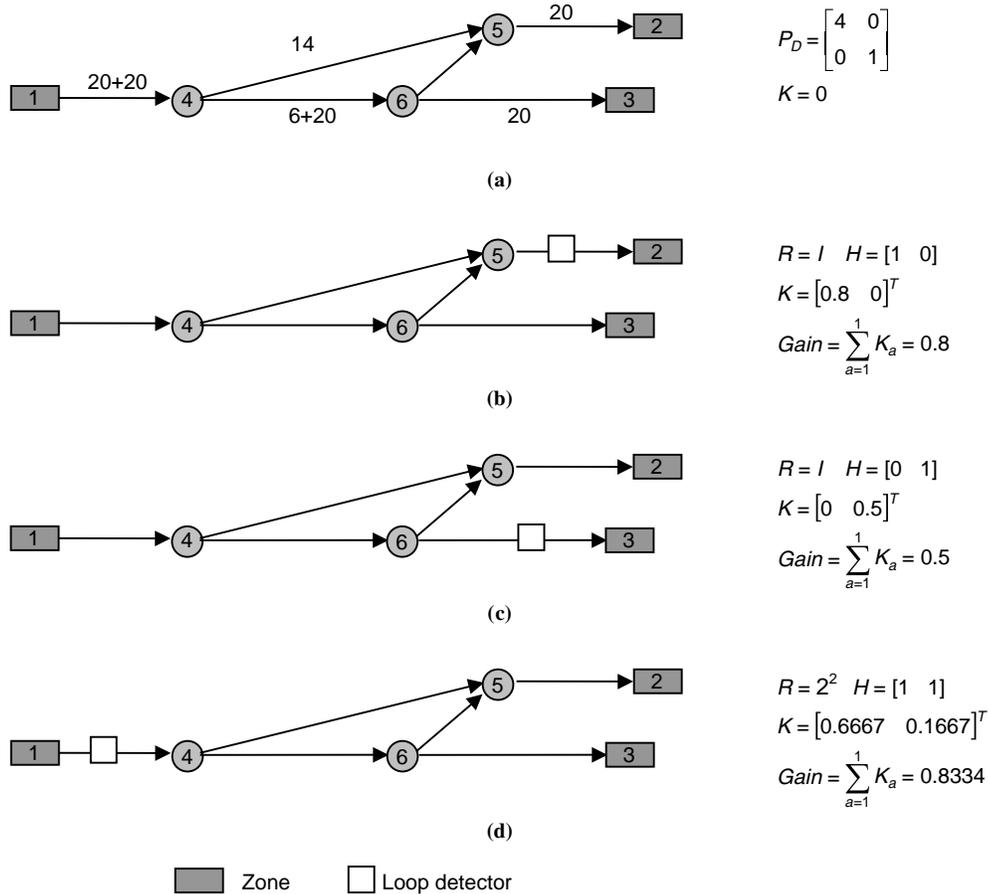
FIGURE 7 Single-point sensor locations: (a) base case, (b) one sensor for O-D pair (1–2), (c) one sensor for O-D pair (1–3), and (d) one sensor for both O-D pairs.
