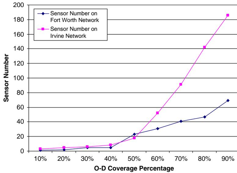
FIGURE 4 Number of sensors needed to cover given percentage of O-D demand.
