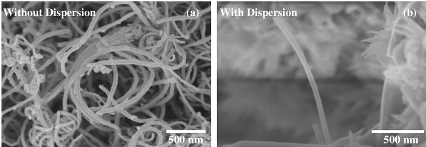
**Fig. 1** SEM images of cement paste reinforced with CNTs dispersed with (FIG. 1(b)) and without (FIG. 1(a)) the application of ultrasonic energy and the use of surfactant
