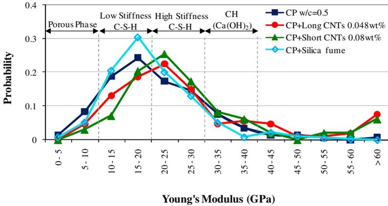
**Fig. 3** Probability plot of the calculated Young's modulus of 28 days cement paste ( $w/c=0.5$ ), cement paste reinforced with 0.048wt% long CNTs, cement paste reinforced with 0.08wt% short CNTs and cement paste with silica fume
