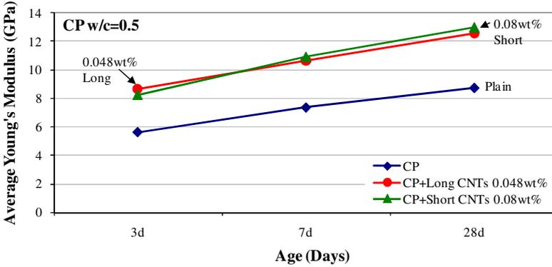
**Fig. 2** Fracture mechanics test results of the Young's modulus of CNTs nanocomposites which exhibit the best mechanical performance among the different mixes tested
