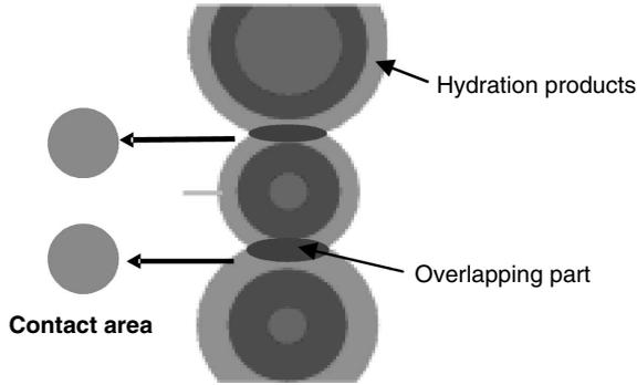
Figure 3. Concept of contact area [11].
