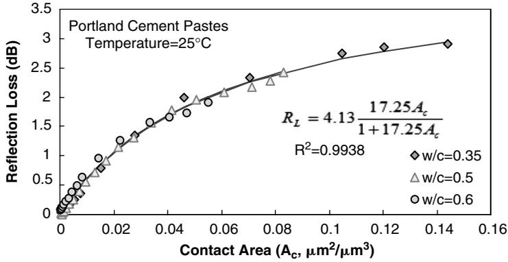
Figure 9. Correlation of reflection loss and specific contact area.
