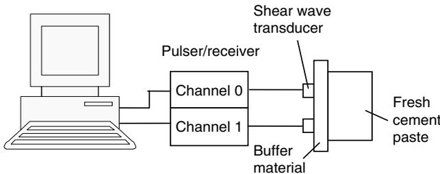
Figure 1. Experimental apparatus for wave reflection measurements.
