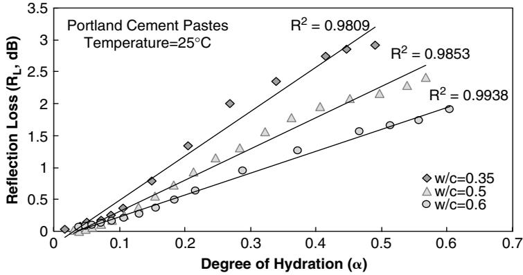
Figure 5. Correlation of reflection loss and degree of hydration.
