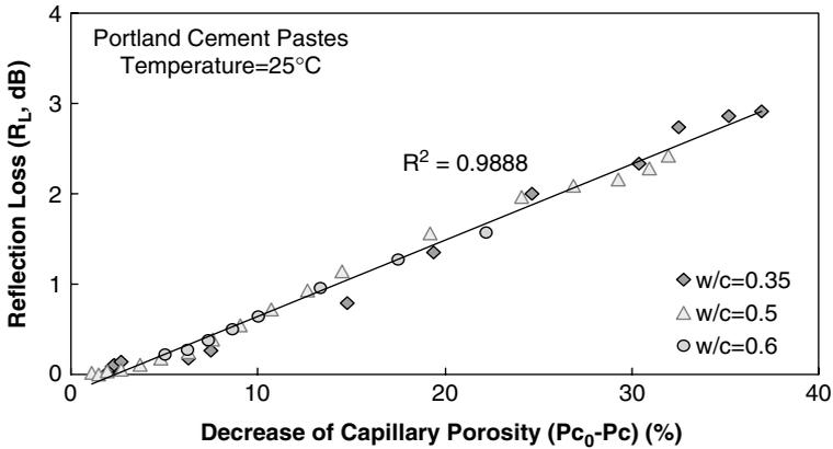
Figure 6. Correlation of reflection loss and decrease of capillary porosity.
