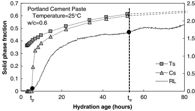
Figure 7. Correlation of reflection loss and solid volume fractions.
