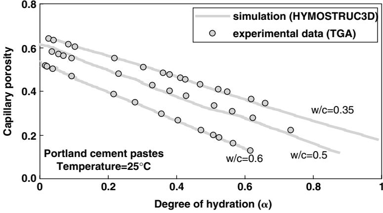
Figure 4. Calibration for degree of hydration and capillary porosity.
