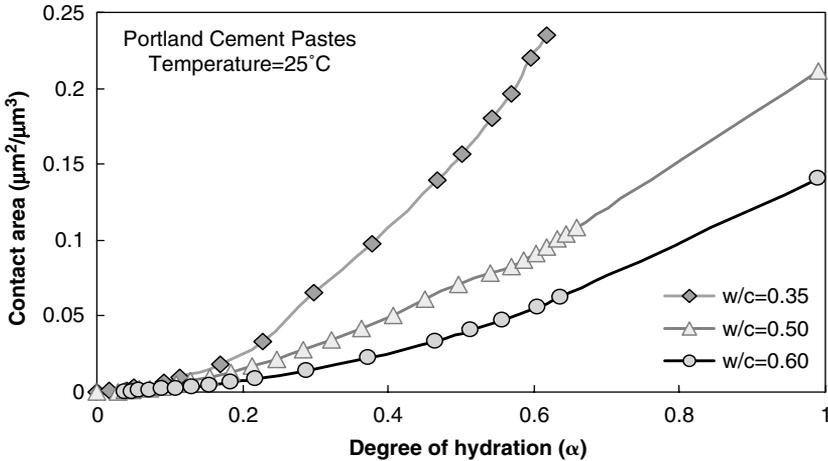
Figure 8. Correlation of specific contact area and degree of hydration.
