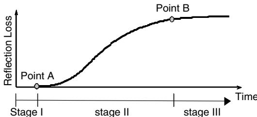
Figure 2. Development of reflection loss of cement paste.
