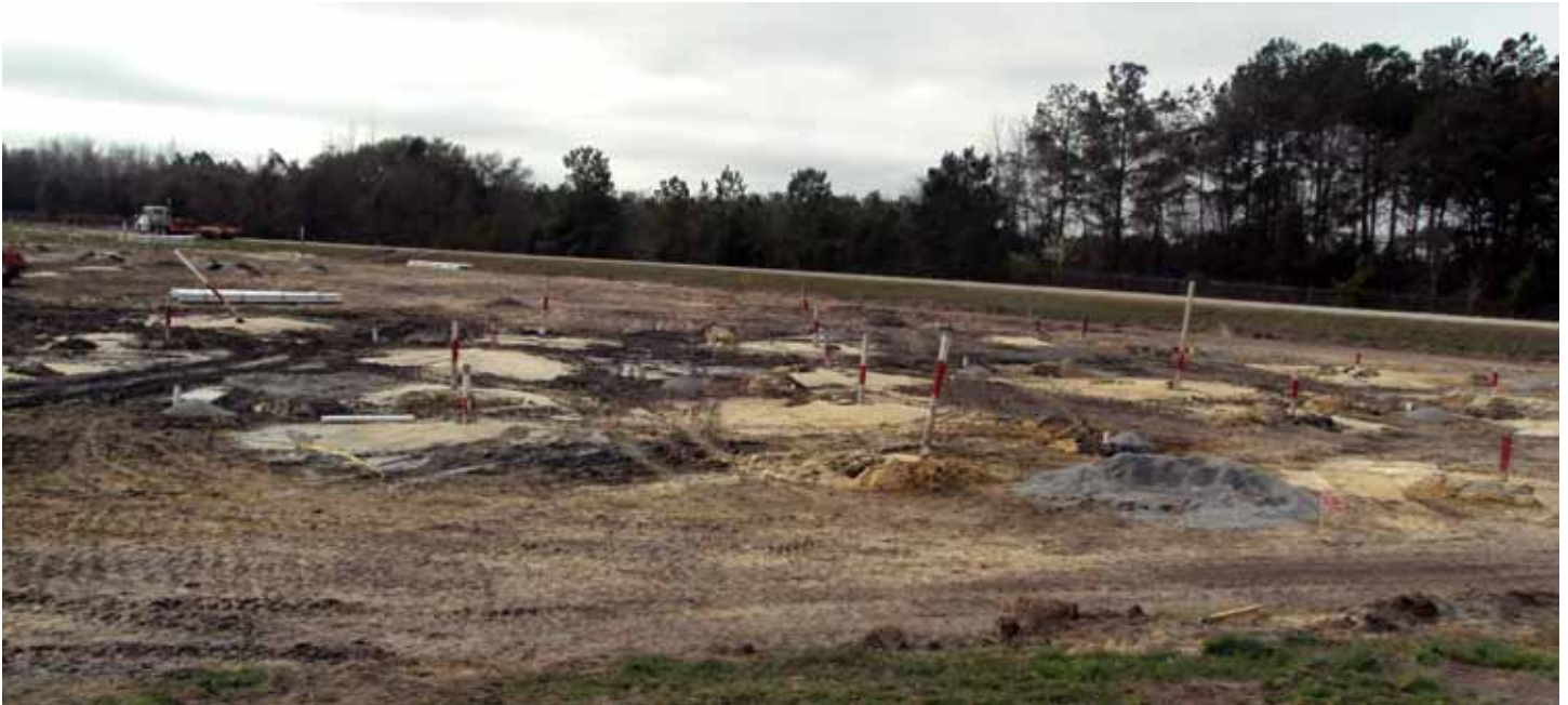
Prof. Finno's team conducted soil tests following blast densification of liquefiable sands at this site in South Carolina.
