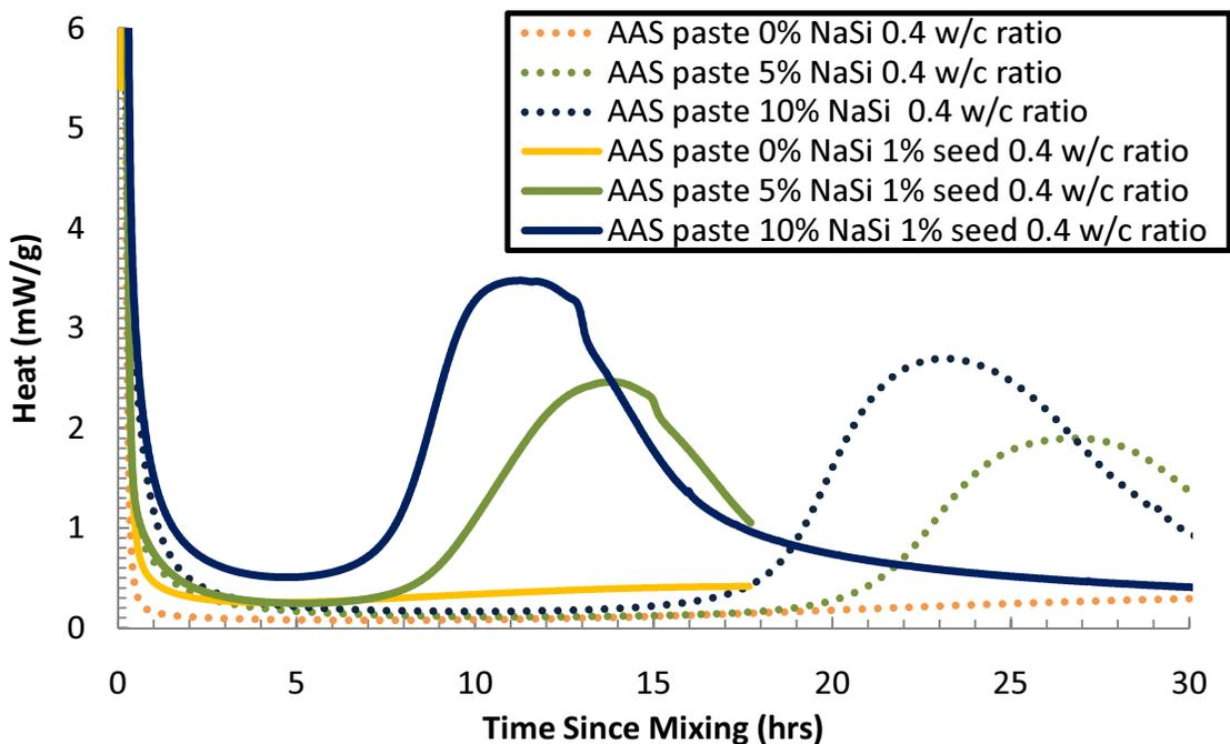
Fig. 1. The heat evolution of activated slag paste with C-S-H seed and either 0%, 5%, and 10% activation by sodium silicate is plotted. The dotted lines indicate the same results for activated slag paste without C-S-H seed.
