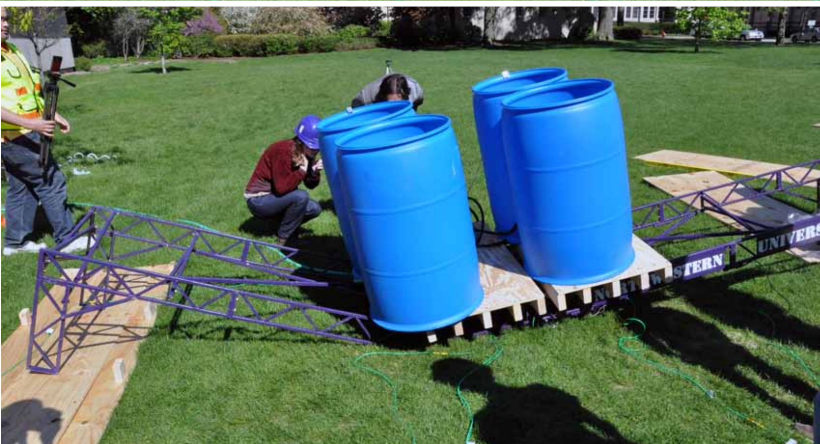
The NU-ASCE students, with the assistance of ITI engineers, load test (to failure) the steel bridge they designed and constructed for the 2011 AISC Student Steel Bridge Competition.
