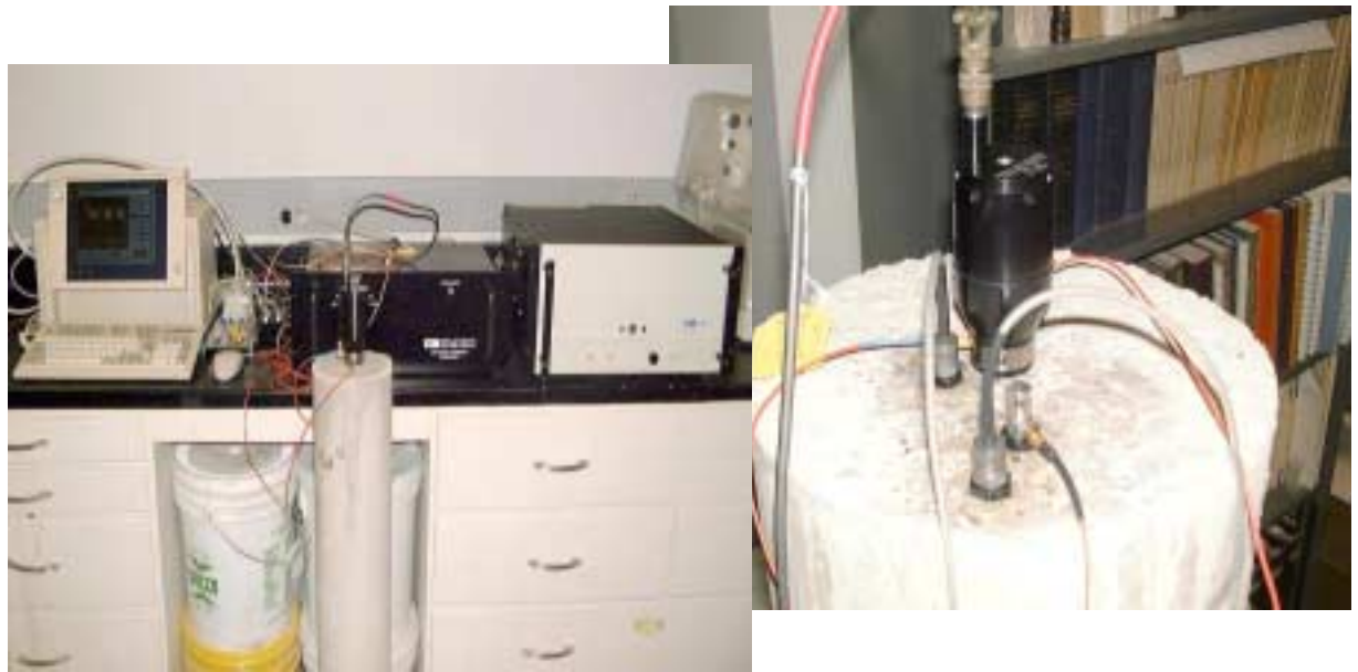
Figure 8. Experimental Set-Up for Guided Wave Tests in Laboratory
