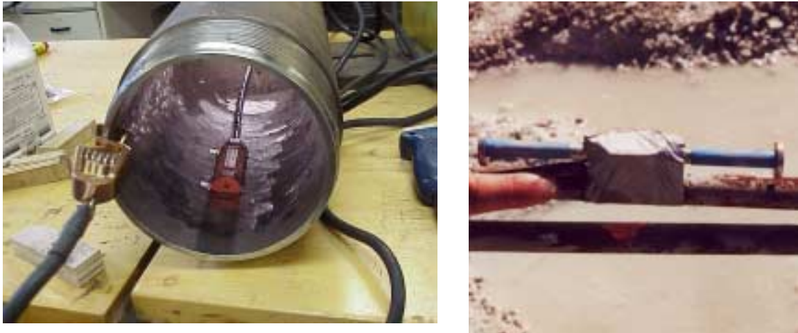
Figure 5. Strain and Embedment Gauges
