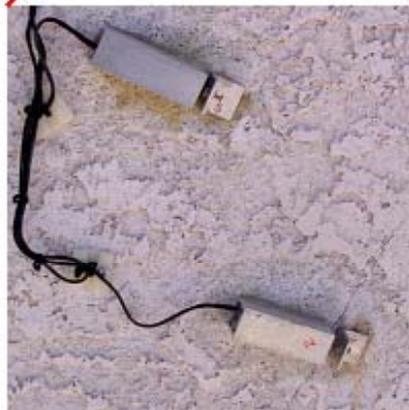
**Photographs of construction and external crack sensor, Top: Trackhoe excavation 12 m from the test house. Middle: Location of external crack sensors on south wall. Bottom: Close-up of external crack and sensors on south wall.**
