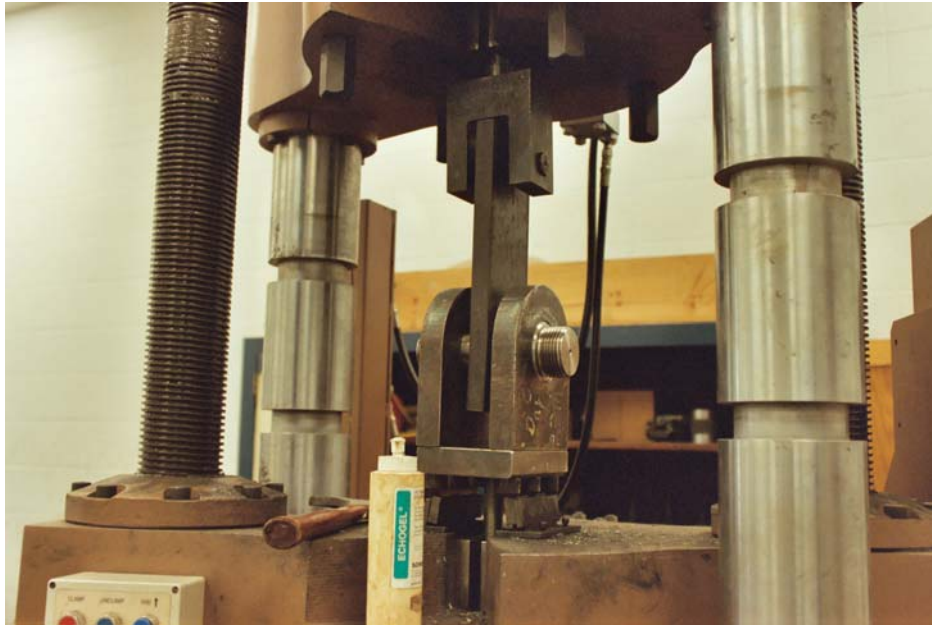
Close up of pin installed in test fixture
