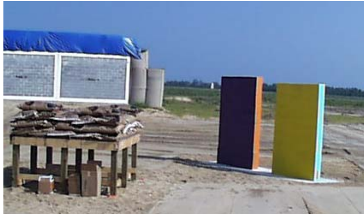
Blast test field at ERDC showing C4 at ground zero and safety concrete and control walls at the right.
