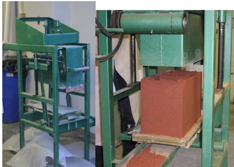
Semi-automatic concrete block making machine (Atlantica Maq, São Paulo, Brazil) used to make safety concrete blocks (left). The mold lists to reveal a freshly made block (made with red dye) sitting on a pallet.
