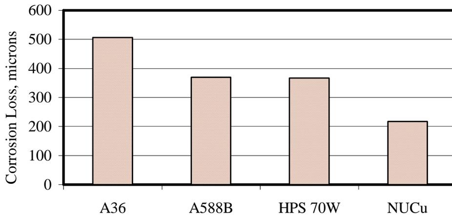
Figure 1. Corrosion loss in accelerated test conducted by Bethlehem
