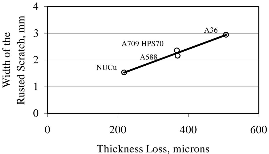
Figure 3. Comparison of the width of the rusted region on the salt sprayed scratched painted steel panels with the thickness loss of the bare steel panels in SAE J2334 tests.
