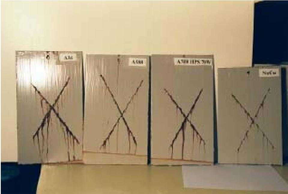
Figure 2. Painted Steel Panels after 3 Weeks, 35°C Exposure in Salt-Fog Chamber (A36; A588; ASTM HPS70W; NUCu (ASTM A710 Grade B) steels)
