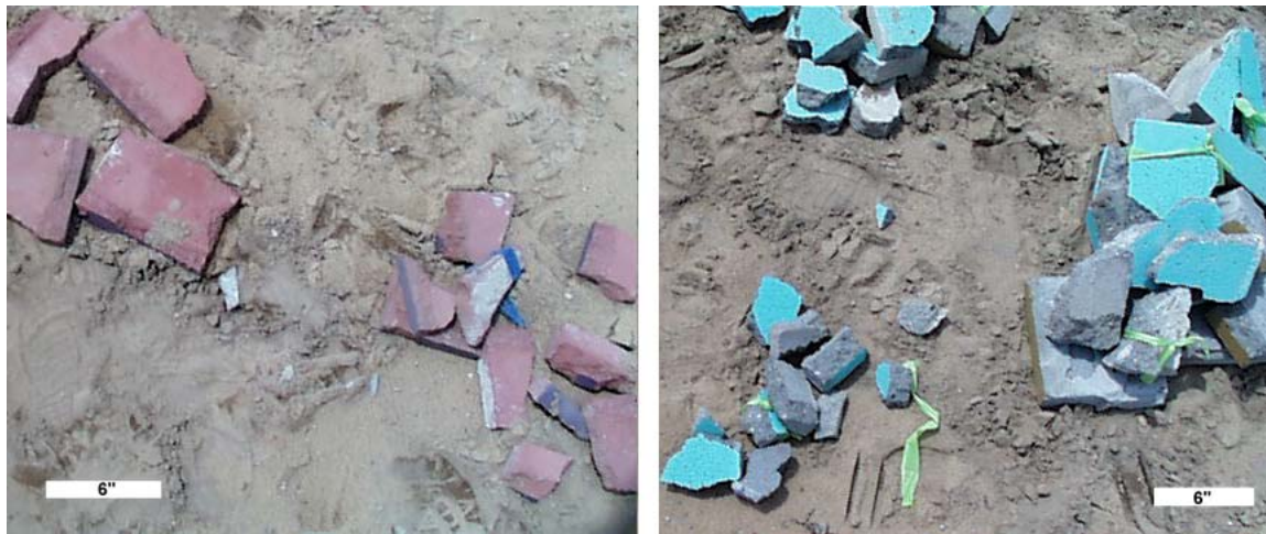
Fig. 6–Fragments from the first field blast: frangible wall left, conventional wall right.
