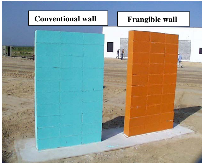
Fig. 3–Test walls ready for field blast experiment.
