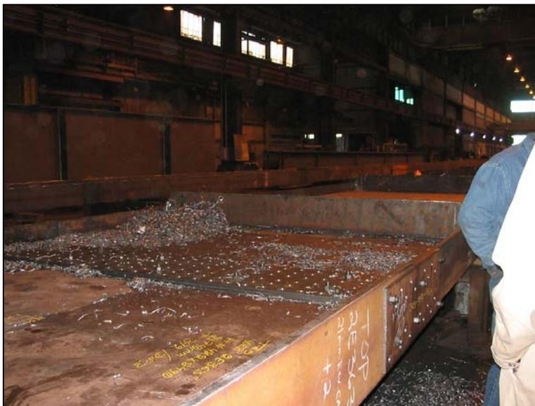
Figure 3. Holes are drilled in girders
