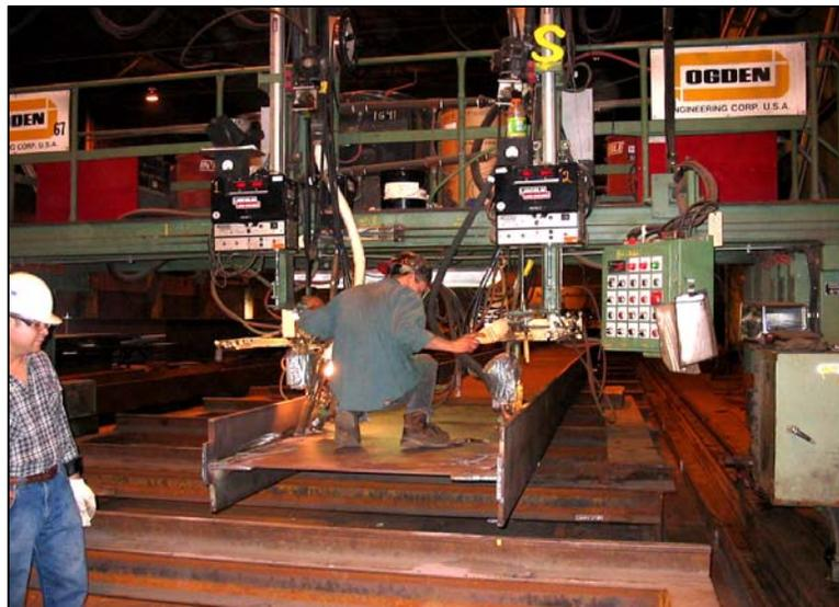
Figure 2. Welding of girders for the Lake Villa bridge at Industrial Steel Construction,
