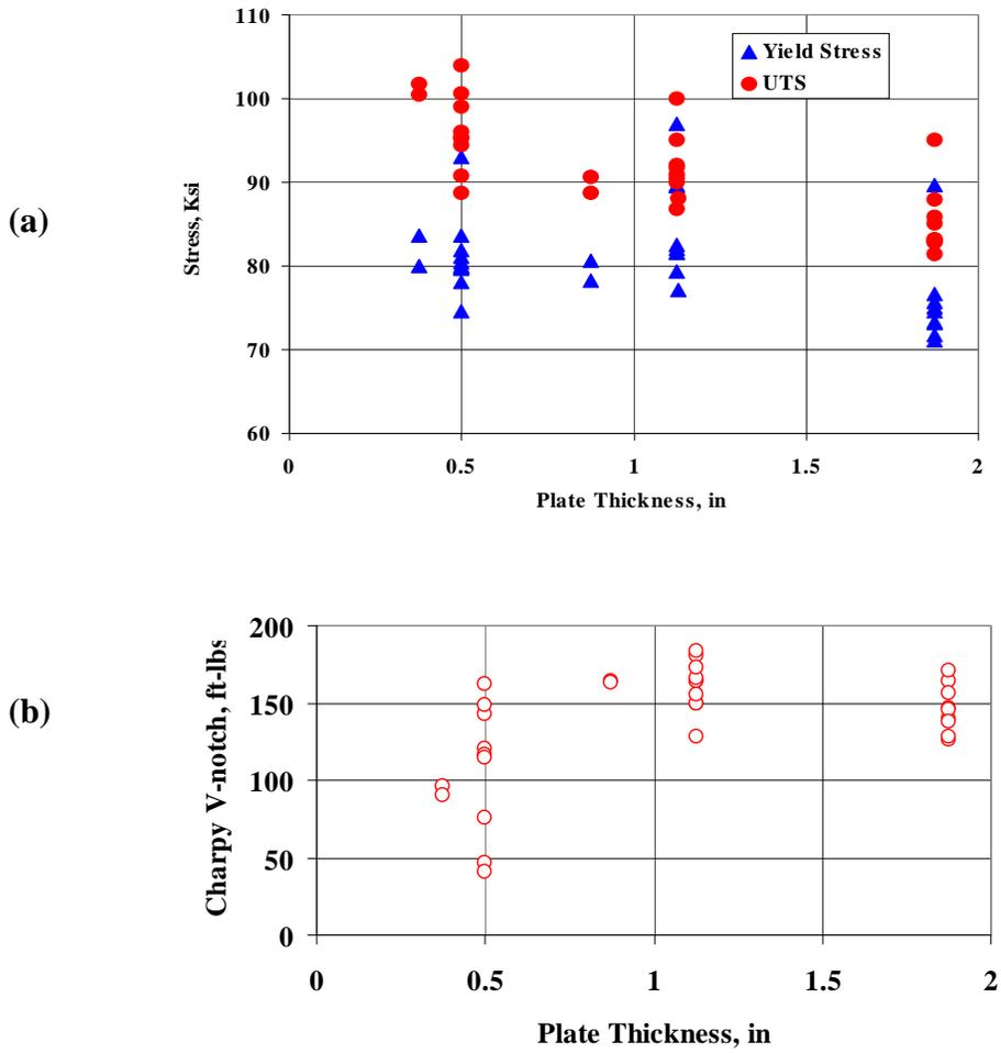
Figure 1. Mechanical properties of A710 Grade B steel used in the Lake Villa, Lake County, IL bridge as a function of plate thickness
