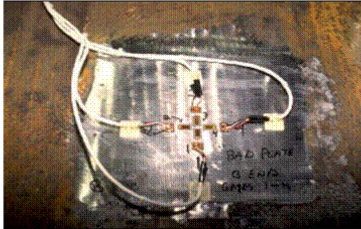
**Figure 3:** Installation pattern of 4 strain gauges at a single location on one of the badly damaged track plates. Photo taken prior to application of weatherproofing layers.
