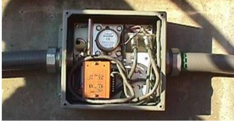
**Figure 8:** Panel box containing a pair of capacitive clinometers for measuring tilt of a pier resulting from scour. Eighteen such boxes were connected to an on-site computer.
